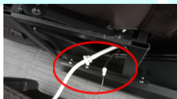
断开气管和端子 Disconnect air hose and terminal
