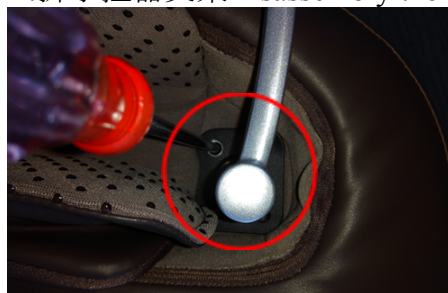
拆除4个固定螺丝 Loose and screw 4screws
