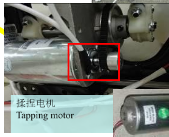
Remove the 2 screws (Lower)
