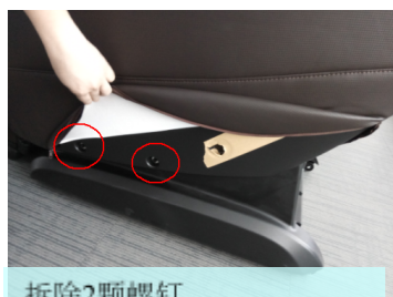
拆除2颗螺钉 Demolition of two screws
