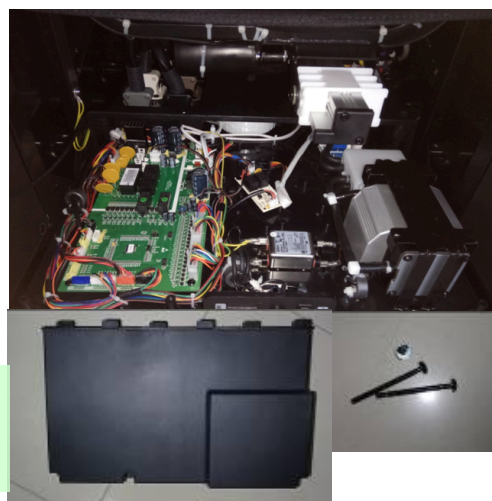
中心盒上前盖上的3枚螺丝 the 3 screws fixing front upper cover for PCB box
