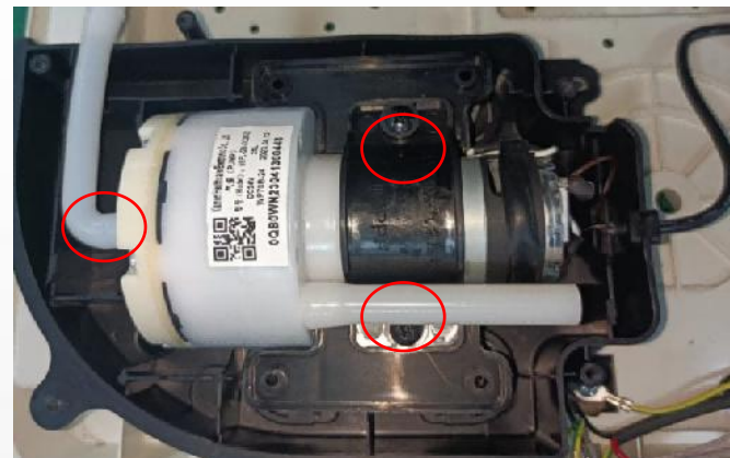
Remove 2 screws, Disconnect the air hose
