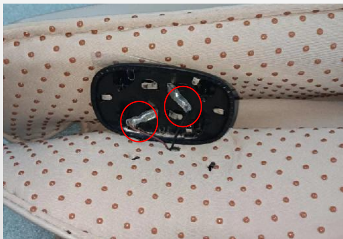
disconnect the signal terminal
