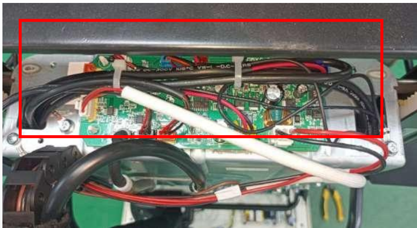
Disconnect the signal terminal
