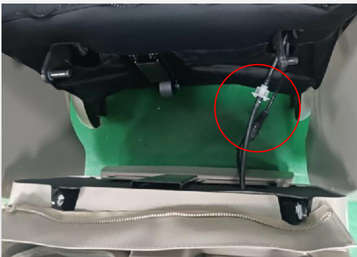
disconnect the air hose and terminals
