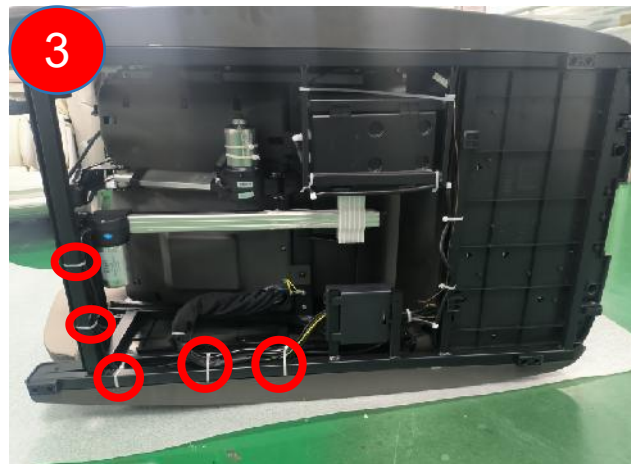
cut the cable tie
