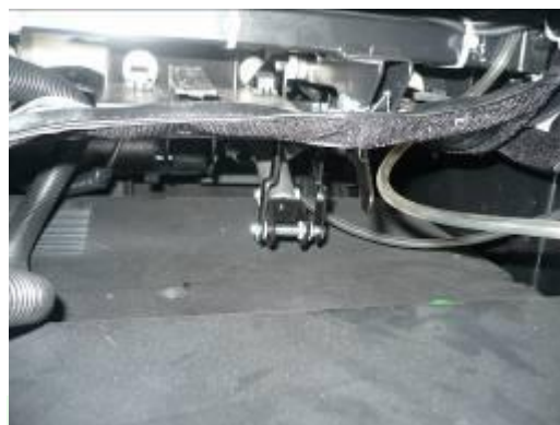
拆卸与连杆连接的销轴 the pin fixing backrest and the actuator
