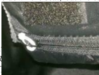
the zipper fixing the seat cover
