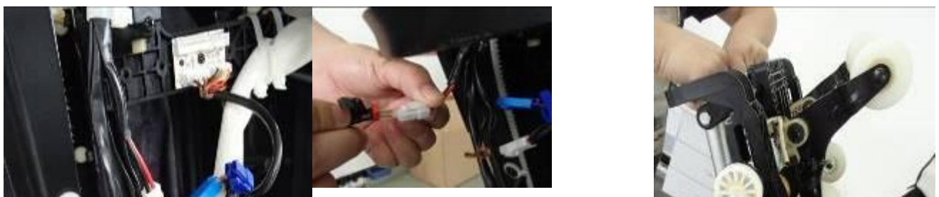
机芯上的电机电源及信号线,请拆除它们 Disconnect moto wire and gear boxsignal , then remove the inner signal later
