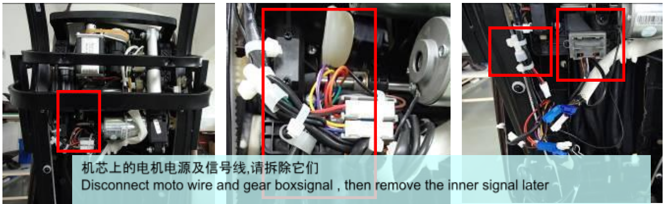
D. 移除机芯上的连接线材 Disconnect the all wire of gear box
