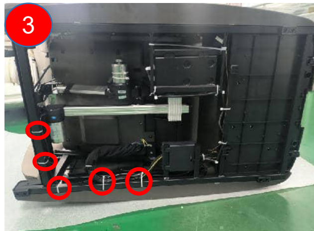
cut the cable tie
