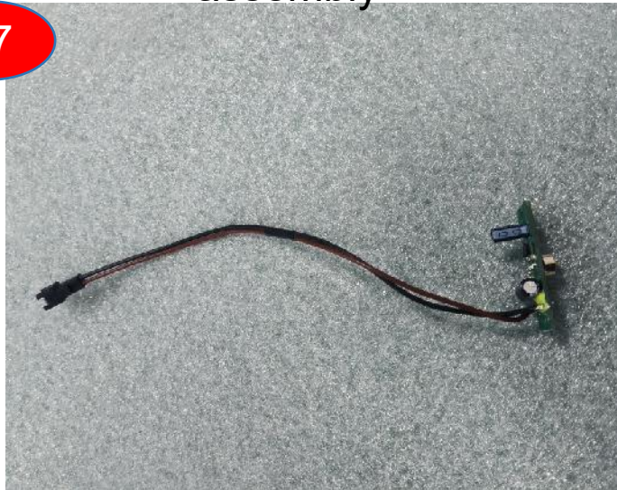
remove charging unit
