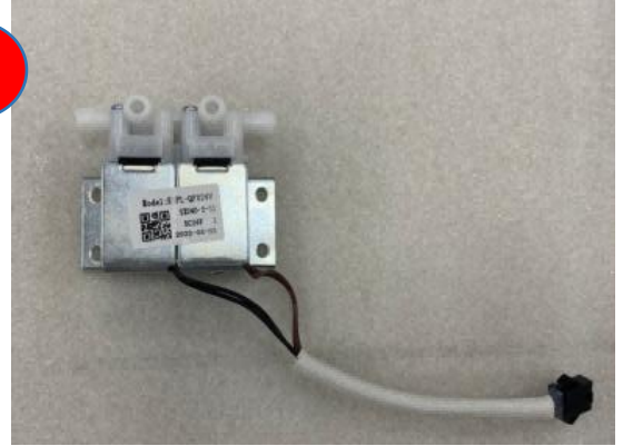
remove the 2-way air valves
