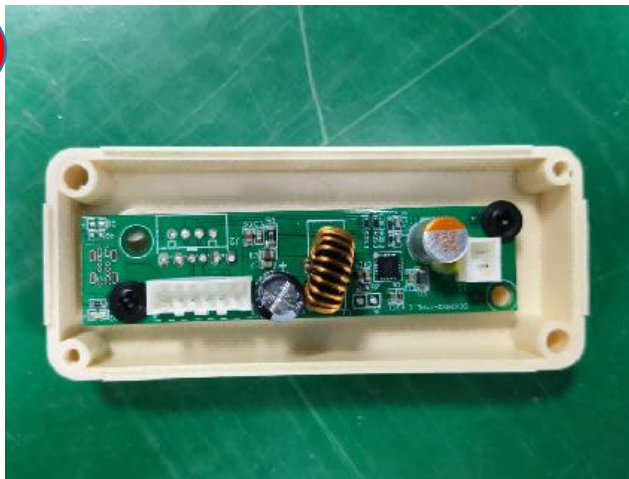
remove the USB charging PCB
