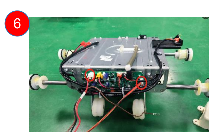
6 disconnect the terminal of the cable tie
