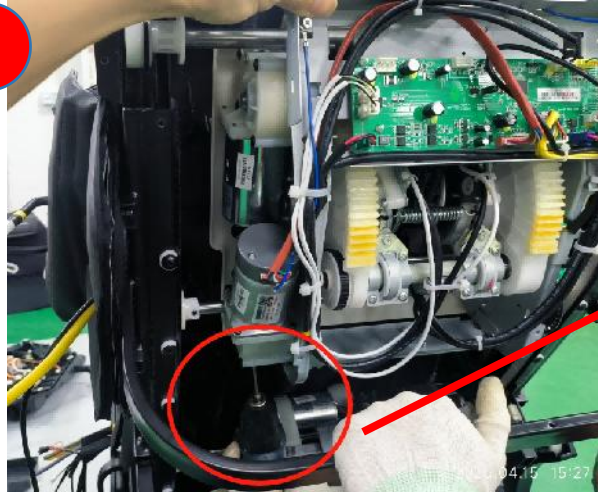
Rotate the rolling motor with a small Phillips screwdriver
