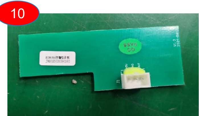
remove collision detection board
