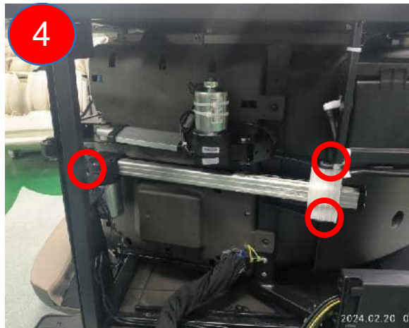
Remove the front pin and rear screw
