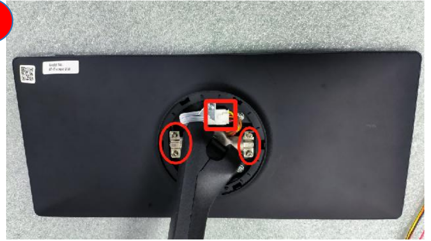
remove the screws, discontent the terminal
