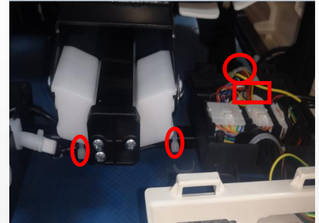
cut the cable tie and discontent the terminal and air hose
