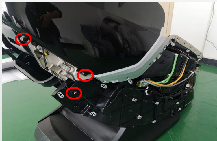
remove 2 screws and discontent the terminal
