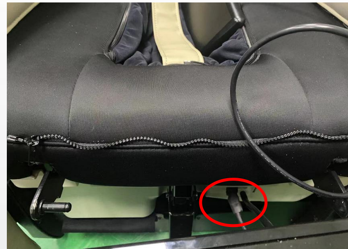
disconnect the terminal and air hose
