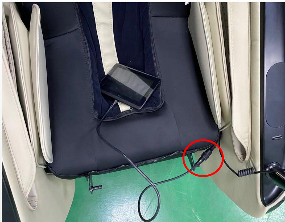
disconnect the terminal
