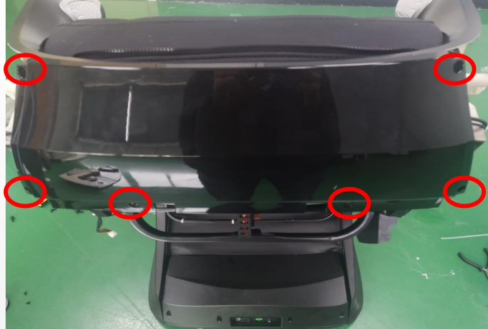
remove 6 screws and remove the cover
