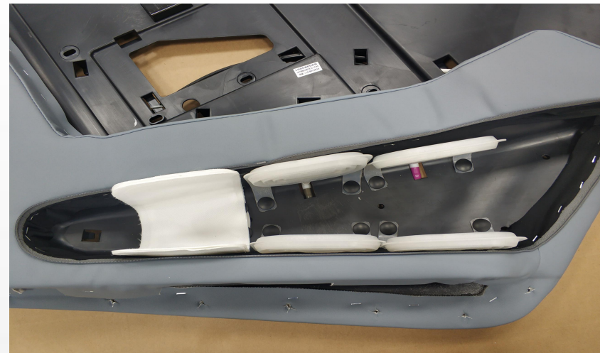
remove the air bag
