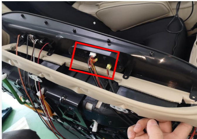
discontent the terminal and remove the cover
