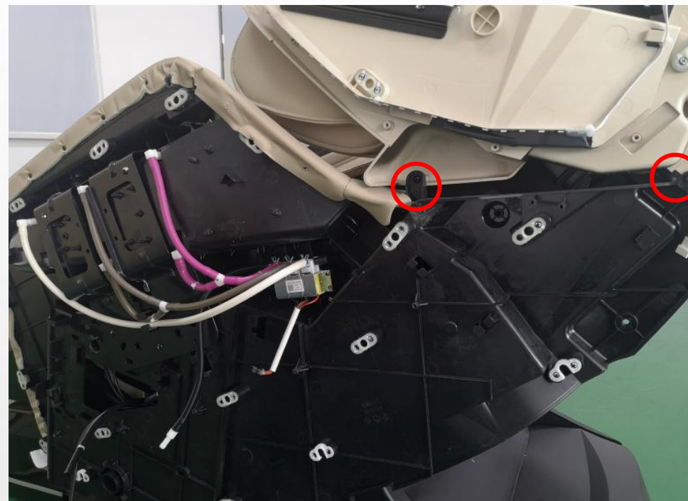
remove 2 screw, then remove left side panel
