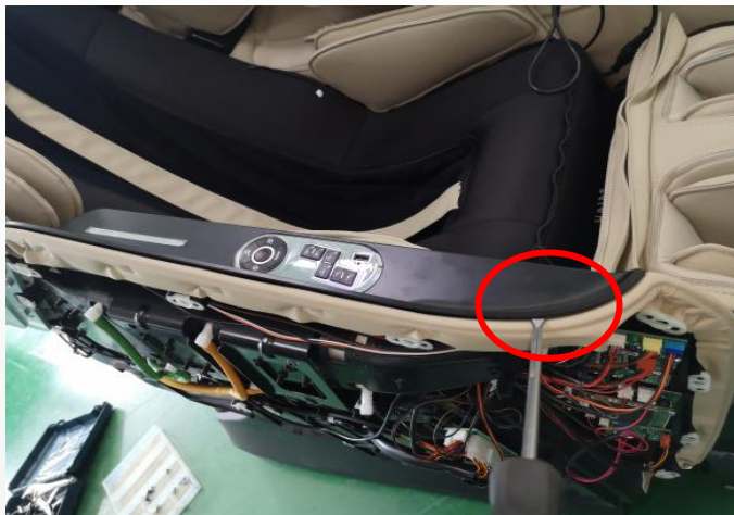
open the cover with a “—” screwdriver
