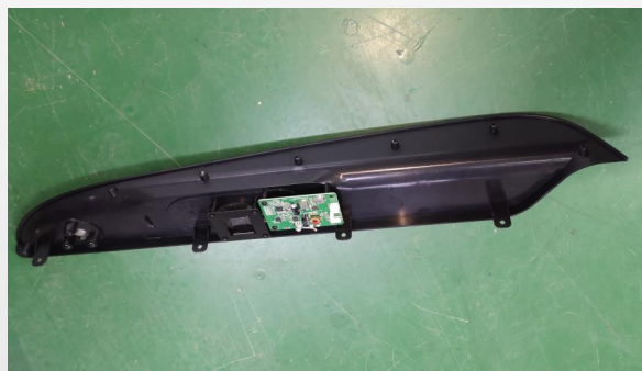
open the cover and discontent the terminals
