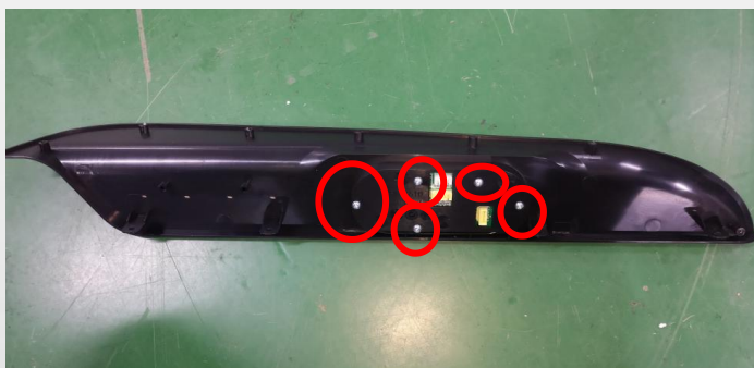
remove 5 screws, remove the control
