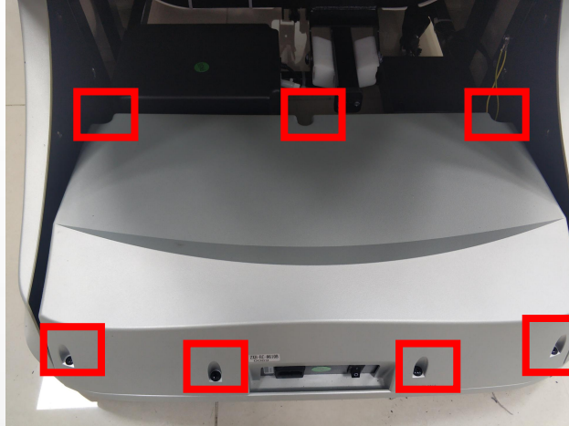
remove 7 screws and remove the cover
