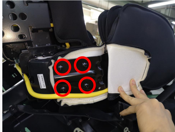
remove 4 screws and remove the shoulder
