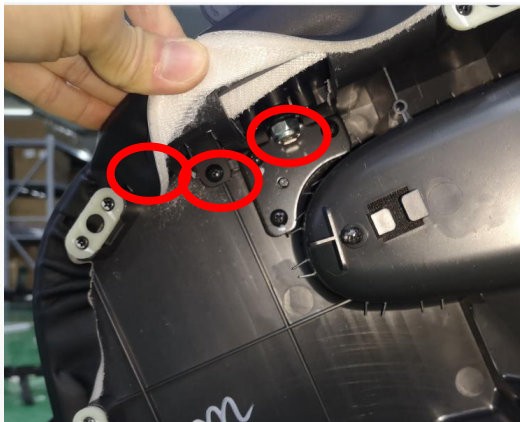
remove the nut and remove the remote control holder
