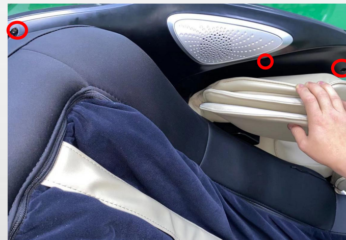
remove 3 screws and remove hood cover
