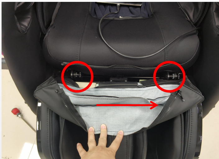
remove 2 baffle, move out legrest towards the right
