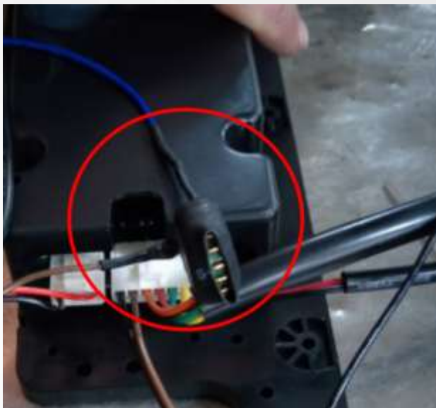
5.剪掉地线, 安装时请对接地线并用电工胶带缠绕 When installing, please connect the grounding wire and wrap it with electrical tape.
