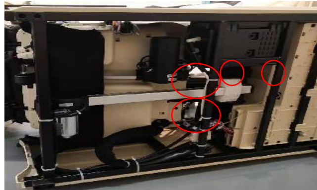
B. cut cable tie, remove 2 screws
