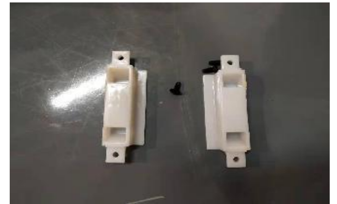
F.Remove the left and right stops of the guide rail
