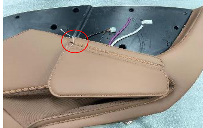
B. separate the leather from plastic screw
