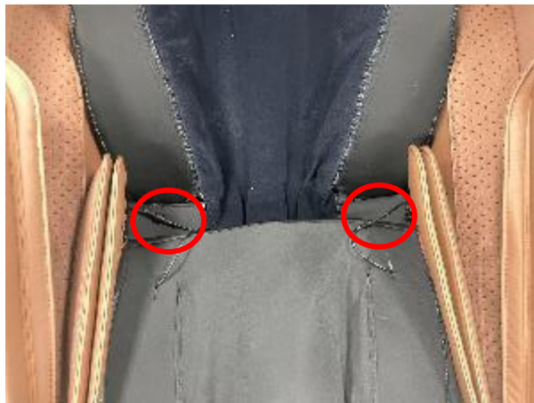
B.Unscrew and unplug 2 heating terminals
