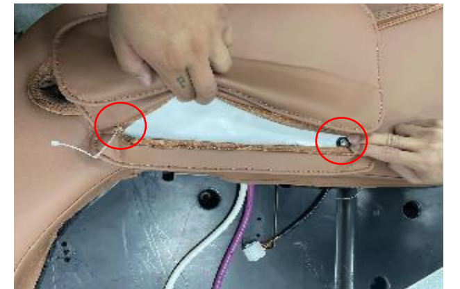
C. remove 4 screws
