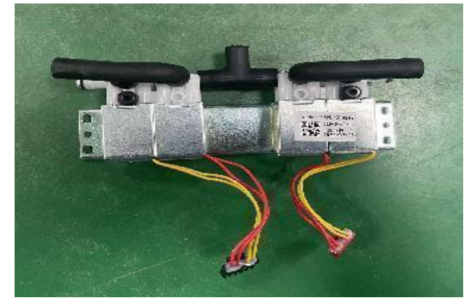
L.remove the air valve
