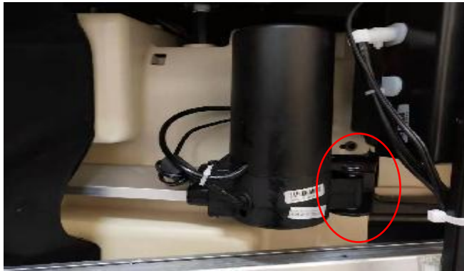
B.cut the cable tie
