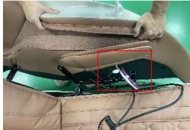
B. disconnect the terminal and air hose
