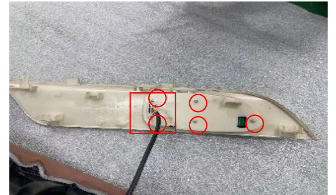
F. remove 5 screws, discontenent the tterminal
