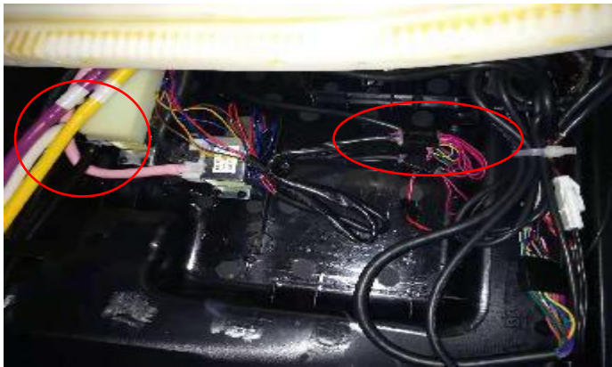
C.disconnect the air hose and terminal
