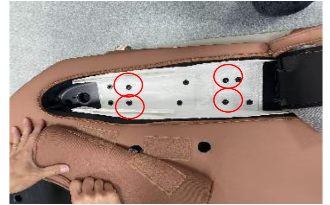
C. remove 4 screws
