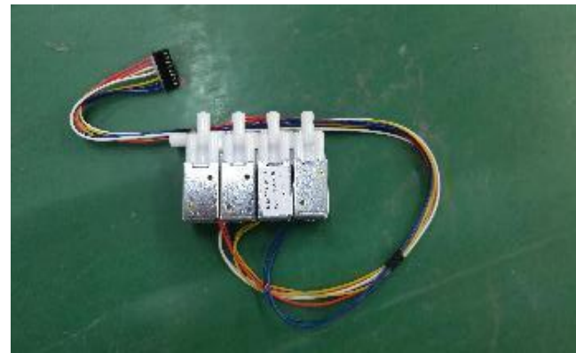
D.remove 4-way air valve
