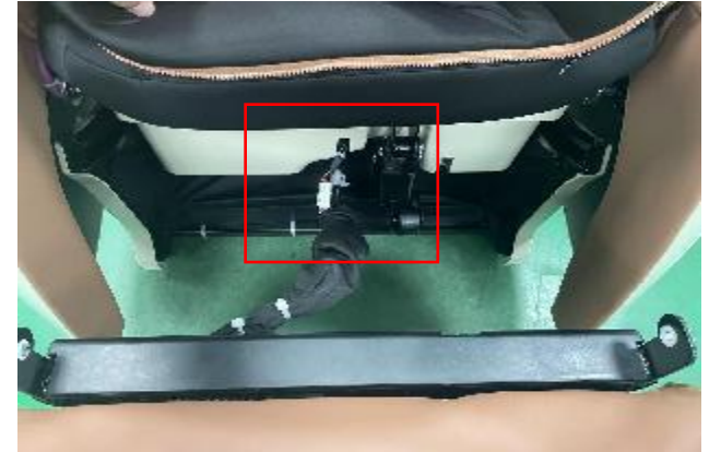
C.disconnect the terminal and air hose
