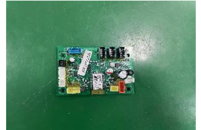
C.remove Bluetooth PCB
