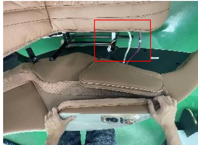
E. disconnect the terminal and air hose
