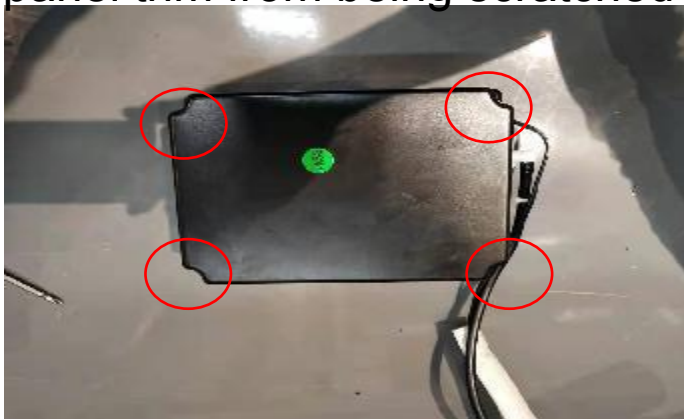
D. remove 4 screws
