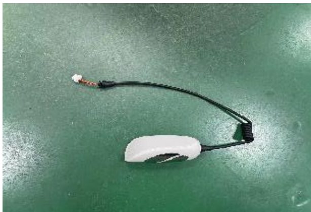
D. remove detection handle
