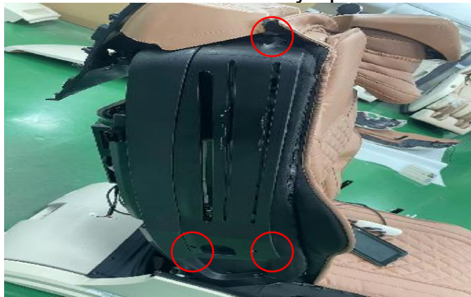
P remove 3 screws
