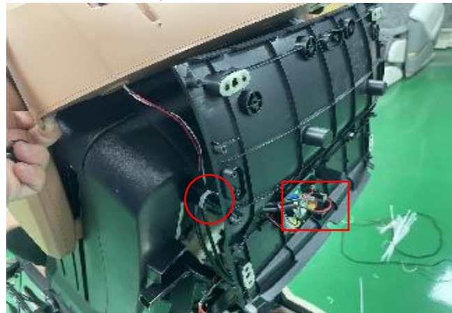
E.cut the cable tie, discontent 2 terminals
