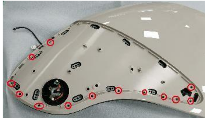
B. Remove 13 screws
