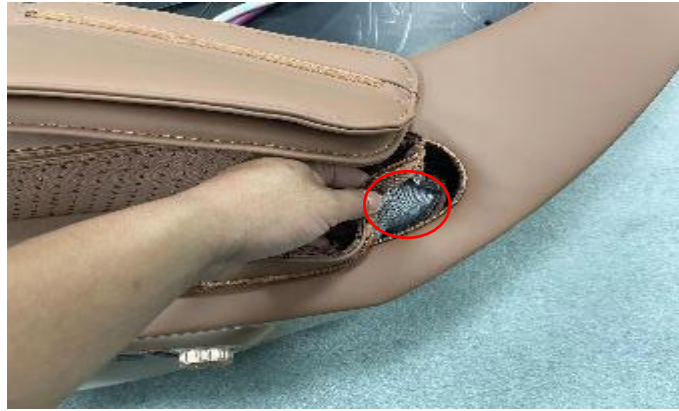
B. separate the leather from plastic screw
