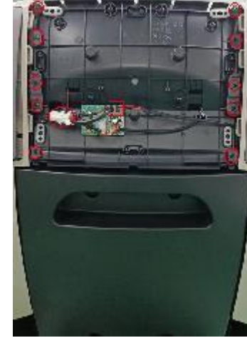
C.Disconnect the port and remove 10 screws
