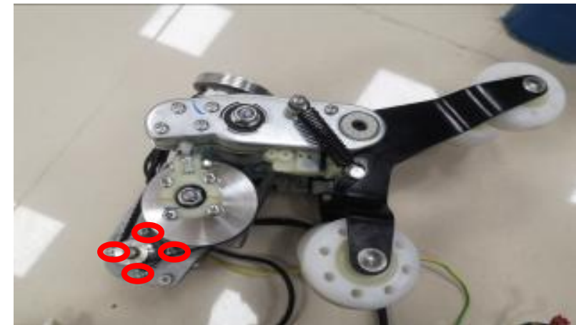
remove 4 screws and take down tapping motor
