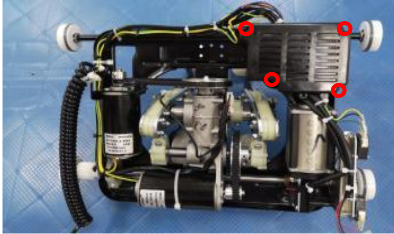
remove 4 screws and open the box
