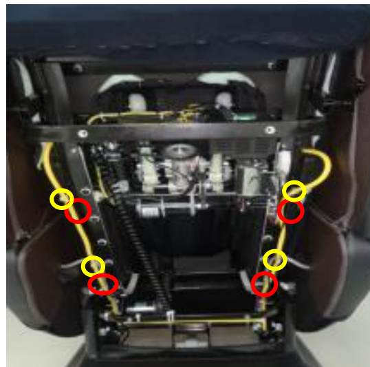
cut the cable tie, disconnect the horn terminal and air hose
