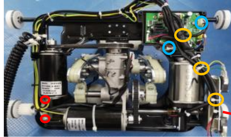
cut cable tie (yellow mark), disconnect 2 terminal (blue mark), remove 6 screws (red mark)
