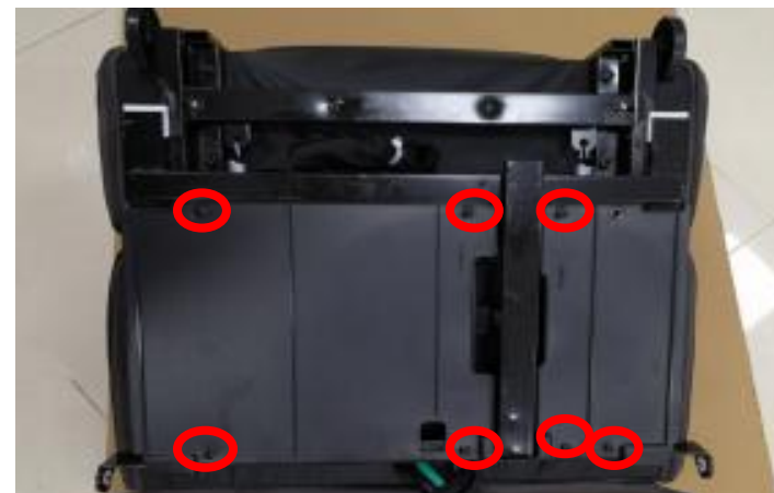
remove 7 screws and take down the cover
