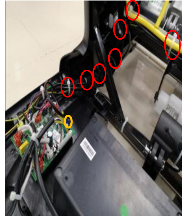
disconnect blue terminal and cut the cable tie (yellow mark), take down the actuator
