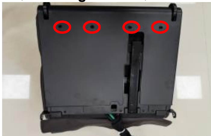
remove 4 screws take down the cover
