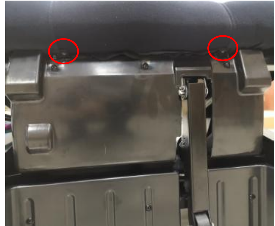
remove 2 screws, now we can take down the front backrest cover
