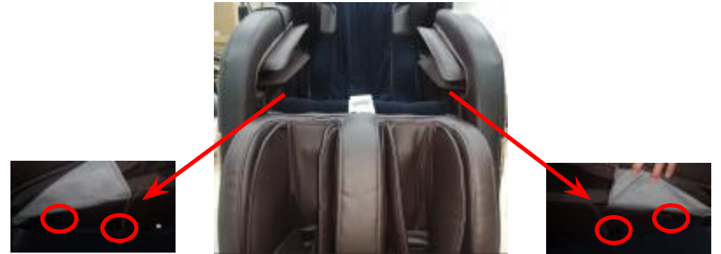
remove 2 screws both side
