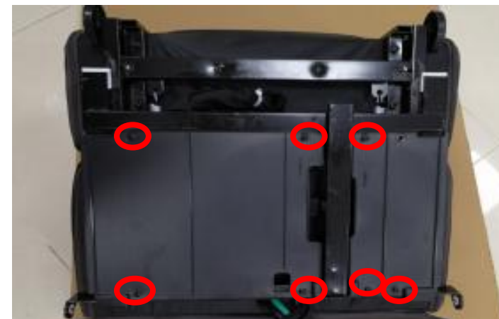
remove 7 screws and take down the cover
