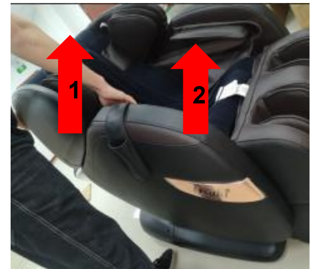
Lift up the side plate according to the sequence 1 and 2 (the sequence marked above), and then remove the side panel
