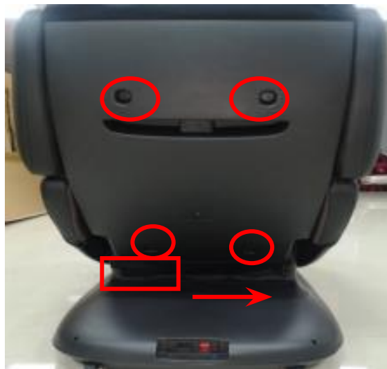
remove the screws and unzip the zipper
