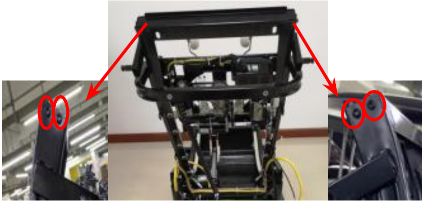
remove 4 screws, take down the frame
