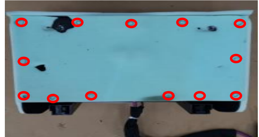
remove 13 screws as the picture marked
