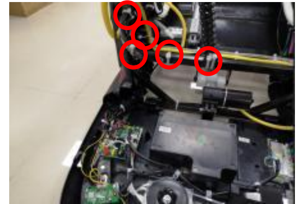
cut the cable tie
