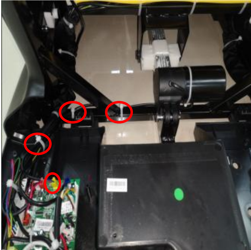
disconnect the yellow terminal and cut the cable tie
