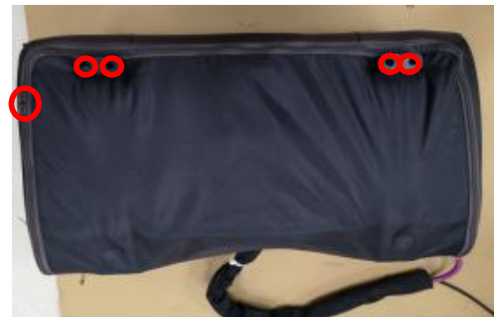
remove 4 screws of the door mat, unzip the zipper, take down the leather
