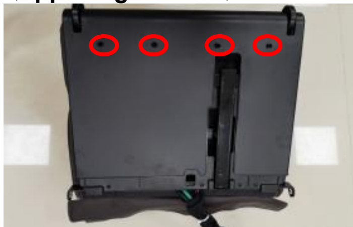
remove 4 screws take down the cover
