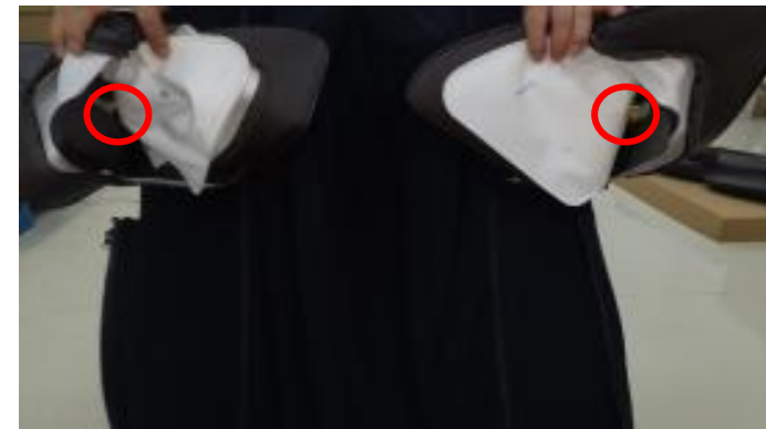
disconnect the air hose and take down the shoulder massage
