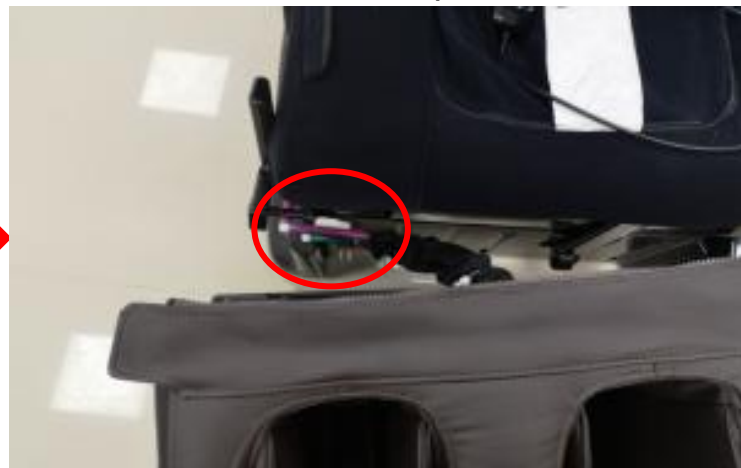
disconnect the air hose and terminals, take down legrest
