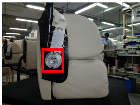
左、右各 3 颗螺丝 Left and right 3 screws
