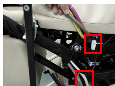
连接线和气管位置 Connecting line and trachea position
