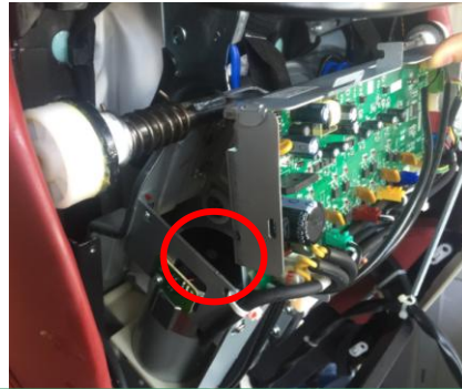
转动行走电机，直到机芯可以脱离背架 Turn motor, until the movement can be separated from the back
