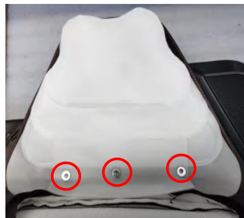
Remove the 3 screws securing the airbag.
