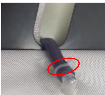
Remove the cable ties and unplug the air tube on the airbag.
