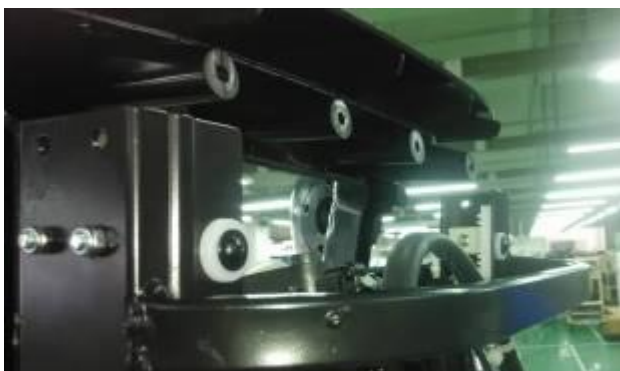
移除靠背顶部的左右防撞块 Remove the 4 screws on top, and then take down the bumper block
