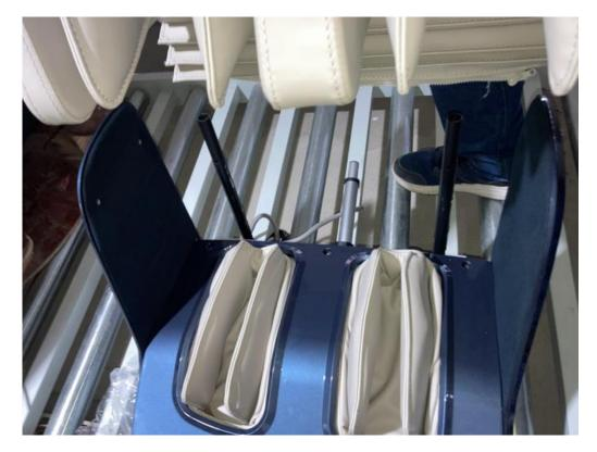
10: As photo below, remove the plastic component on footrest with a plastic crowbar ;
