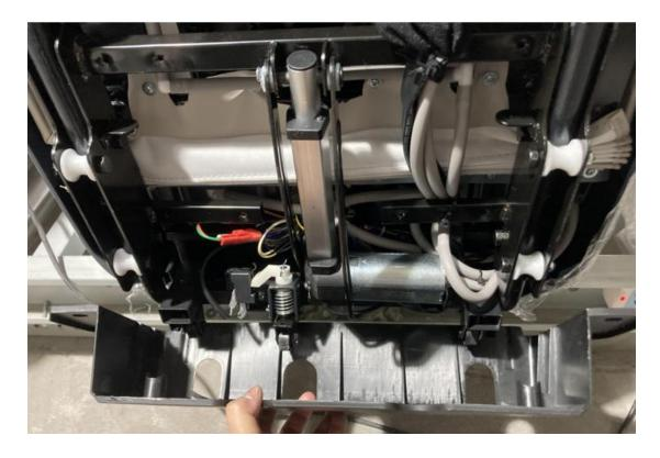
: As photo below, remove the R- shaped bolt in the joint;
