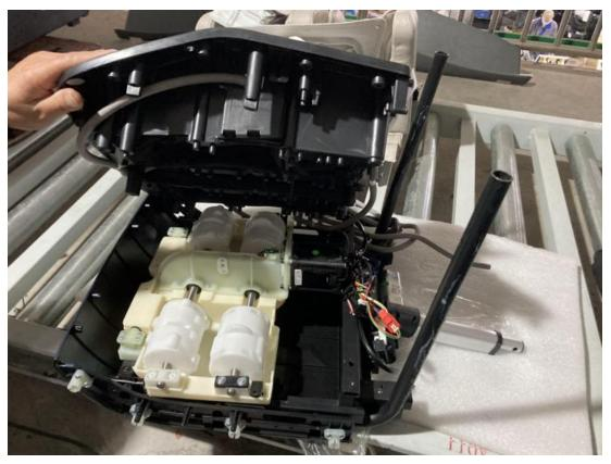
21: As photo below, remove all the screws on both side;
