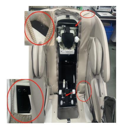
2: As photo below, disconnect the cable connector and air pipe joint in side panel;
