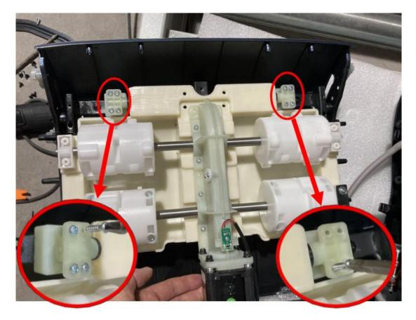
22: As photo below, devided the cable of the foot roller moter.
