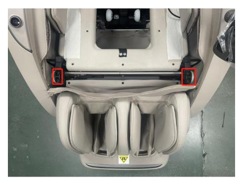
2: As photo below, disconnect the cable connector and air pipe joint;
