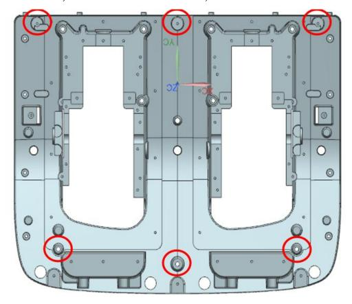
20: As photo below, plastic cover can be devided after unscrewing .
