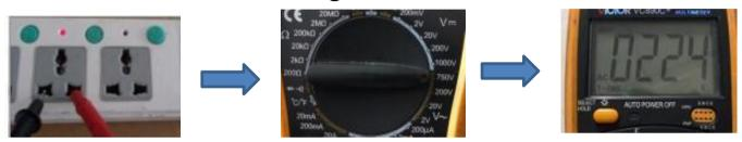
As shown in the picture above: measure the household plug-in board power supply (220V), select the range of 750, and the test result shows "224", indicating that the actual voltage of this group of sockets is 224v at the moment (the switch is pressed down, so there is power, and the light is on).
