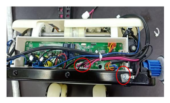
discontent the white terminal, remove the screw, separate the backrest wire, let mechanism go up with 24V/DC power
