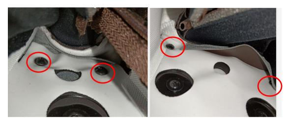
remove 4 screws fixing the air bag
