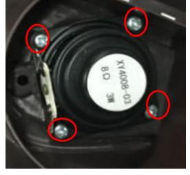
Remove four screws and replace the horn
