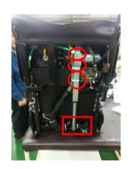
cut the cable tie, take down the shaft
