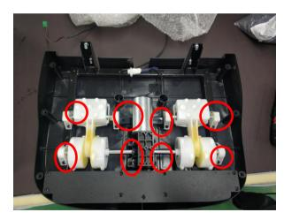
remove 16 screws separate the foot massage
