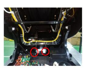
remove 2 screws fixing the actuator
