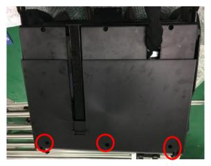
remove 3 screws fixing the rear cover
