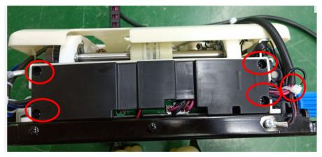
remove 4 screws, cut the cable tie
