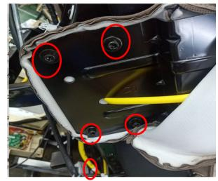
discontent the air hose, remove 4 screws
