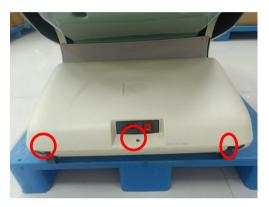
remove 3 screws, remove the cover
