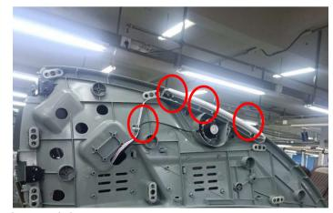
cut the cable tie, remove 3 screws
