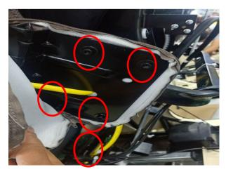
discontent the air hose, remove 4 screws
