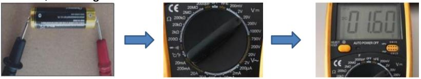
As shown in the picture above: the test result is "1.58", indicating that the voltage at both ends of the battery is 1.58v, and the red lead is connected to the "+" pole of the battery, and the black lead is connected to the "-" pole of the electromagnetic.
