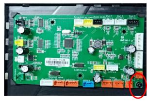
remove the screw and remove main PCB
