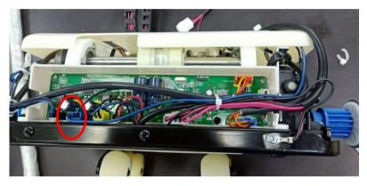
find out the blue terminal, let mechanism go down with 24/DC power
