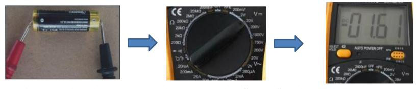
As shown in the above picture: the test result is "- 1.58", indicating that the voltage at both ends of the battery is 1.58v, and the red lead is connected to the "-" pole of the battery, and the black lead is connected to the "+" pole of the electromagnetic
