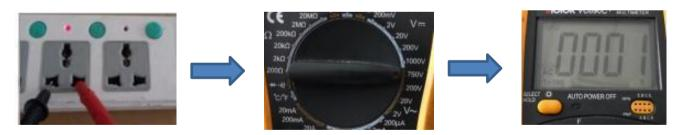
As shown in the above picture: measure the power supply (220V) of our household plug-in board, select the range of 750, and the test result is displayed as "001", indicating that the actual voltage of this group of sockets is 0V at the moment (the switch is not pressed down, so there is no power, and the light is not on).
