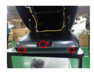
remove 3 screws fixing main PCB box
