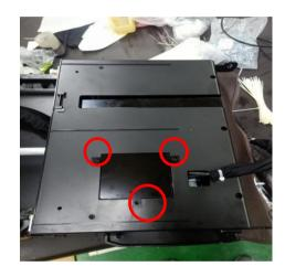
remove 3 screws fixing the box
