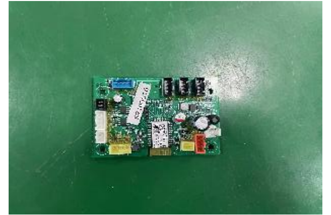
C.remove Bluetooth PCB
