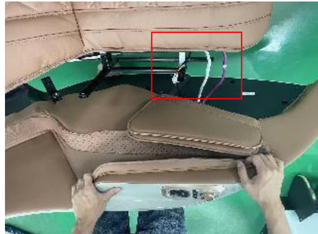
E. disconnect the terminal and air hose
