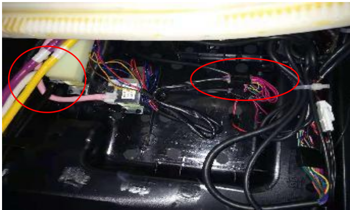
C.discontent the air hose and terminal
