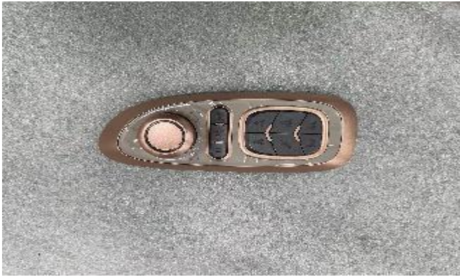
G. remove the side panel control
