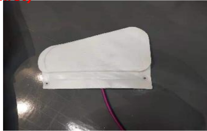
H .remove the air bag
