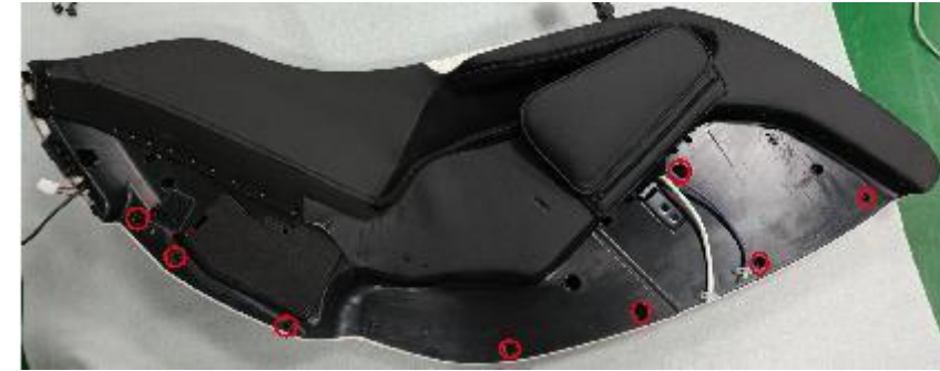
C. Remove 8 screws
