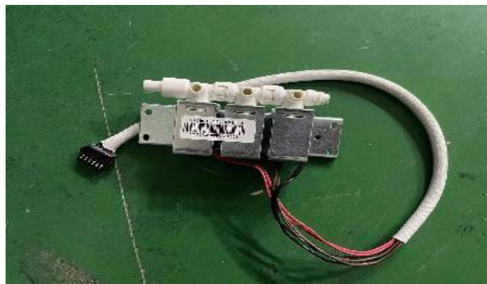
K.remove the 3-way air valve
