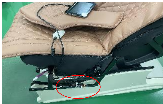
B.cut the cable tie
