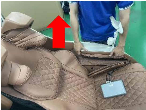
D. Extract right side panel upwards
