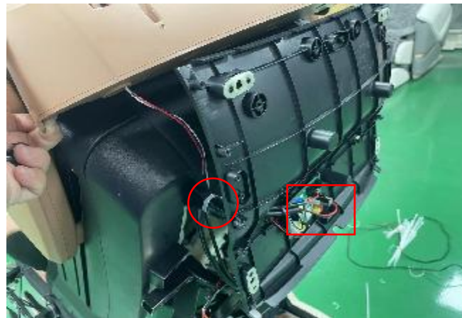
E.cut the cable tie, discontent 2 terminals
