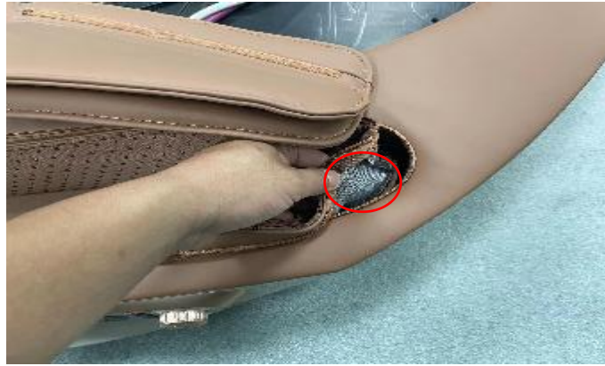
B. separate the leather from plastic screw
