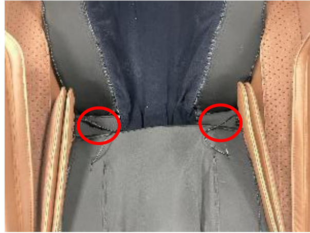
B.Unscrew and unplug 2 heating terminals
