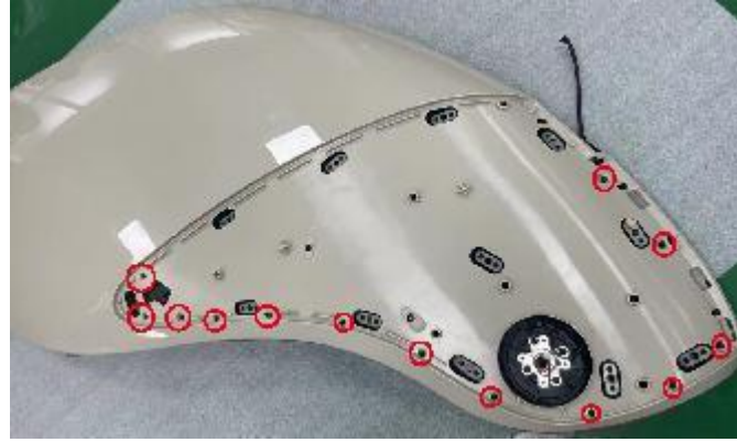
B. remove 13 screws
