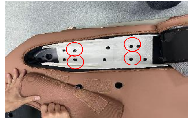
C. remove 4 screws
