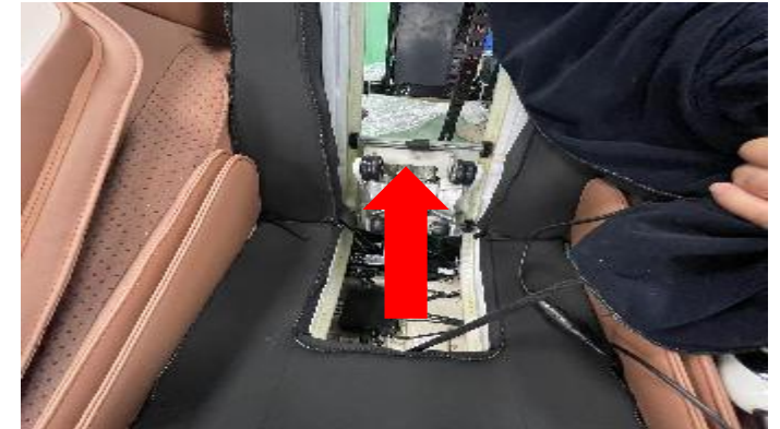
C.Push the mechanism upward to an appropriate angle by hand
