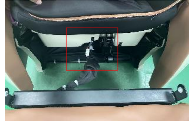
C.disconnect the terminal and air hose
