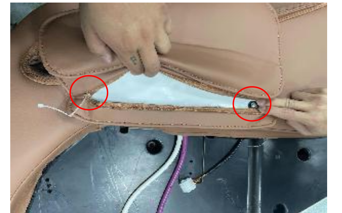
C. remove 4 screws
