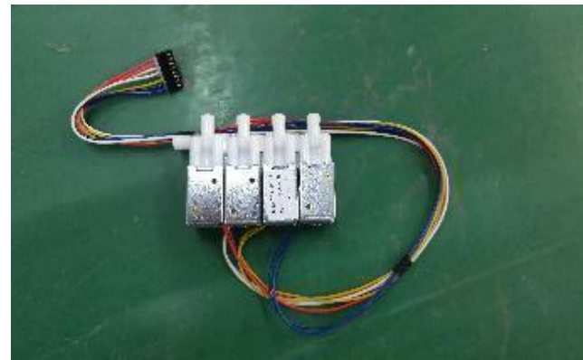
D.remove 4-way air valve
