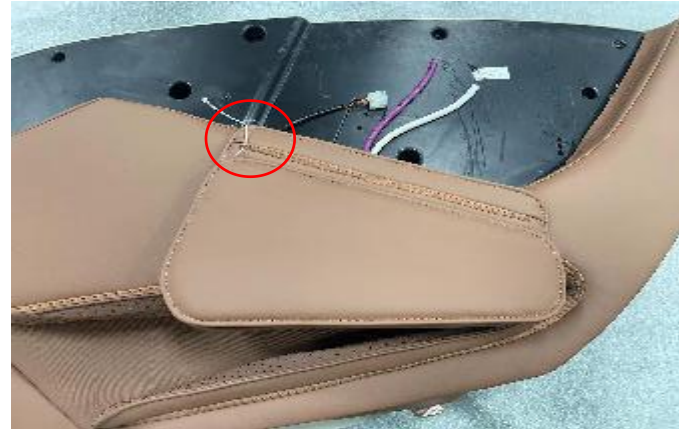
B. separate the leather from plastic screw
