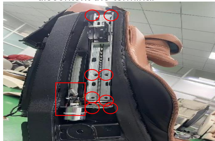
Q .remove 8 screws, cut the cable tie and disconnected the terminal
