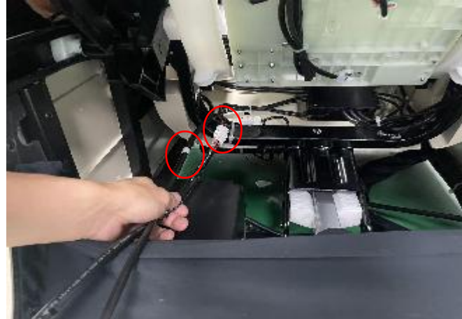
H.disconnect the terminal and air hose
