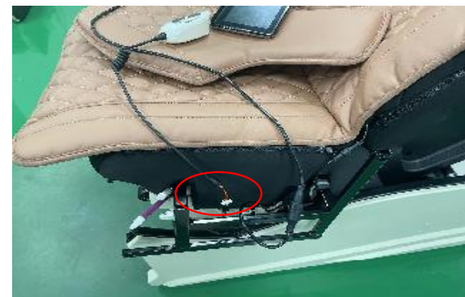
C. disconnected the terminal
