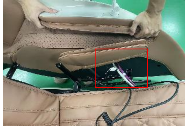
B. disconnect the terminal and air hose
