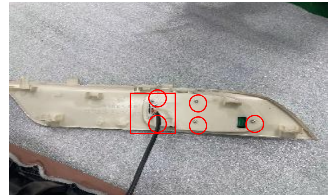
F. remove 5 screws, discontent the tterminal
