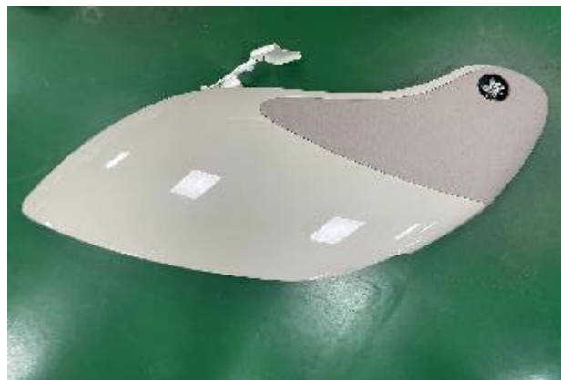
A.remove left side panel
