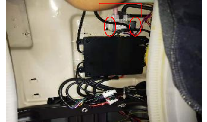
C.remove the screws, disconten the terminals, remove air valve
