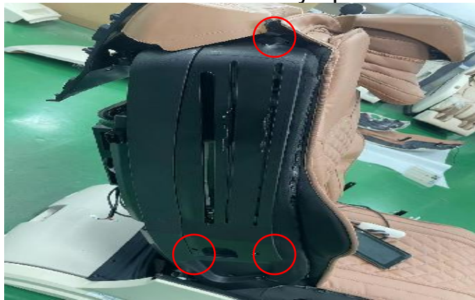
P remove 3 screws
