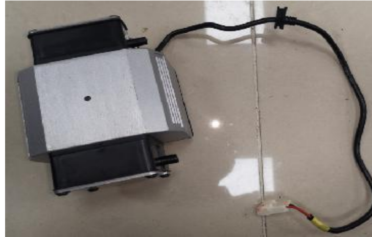
H.remove air pump
