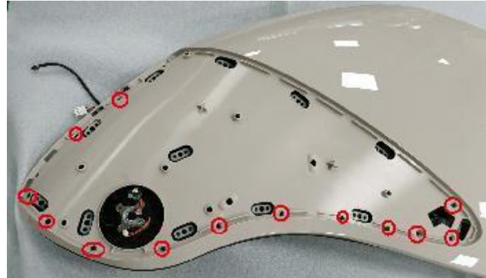
B. Remove 13 screws
