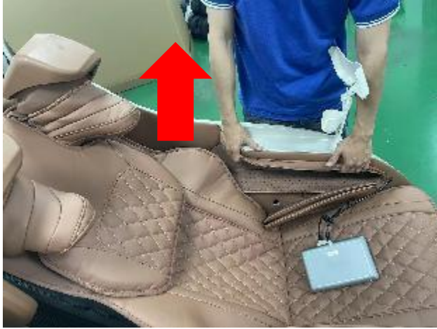
A. Extract left side panel upwards
