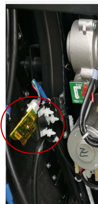
2. Take off the Upper Limit Sensor Detection Board, but do not unplug it.
