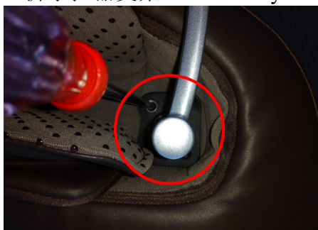
拆除 4 个固定螺丝 Loose and screw 4 screws
