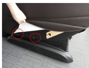
拆除 2 颗螺钉 Demolition of two screws
