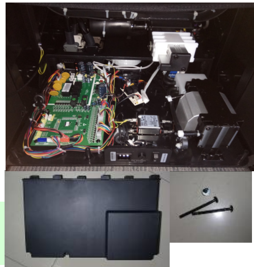
中心盒上前盖上的3枚螺丝 the 3 screws fixing front upper cover for PCB box
