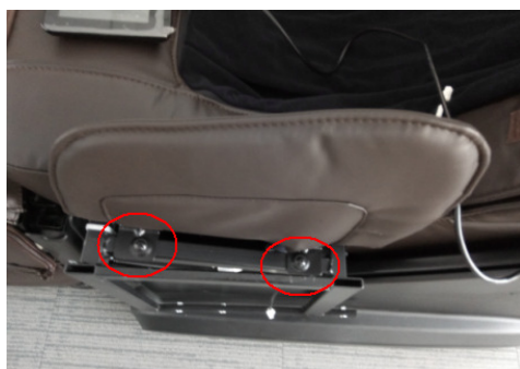
拆除 2 颗螺钉 Demolition of two screws
