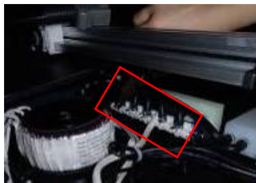
取下固定气阀的四枚螺丝，拔掉接线端子，可以更换气阀 Slack and remove the 4 screws, disconnect the terminal of the air valve
