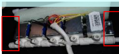
取下固定气阀的四枚螺丝，拔掉接线端子，可以更换气阀 Slack and remove the 4 screws, disconnect the terminal of the air valve
