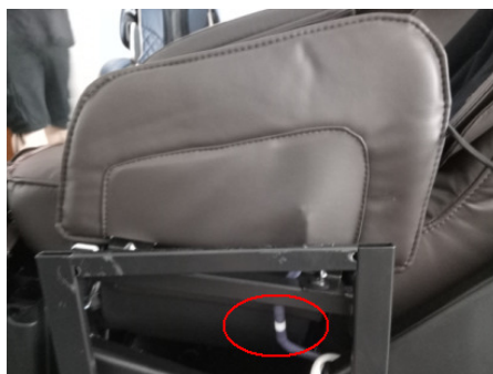
断开气管 Disconnect terminal
