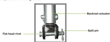
• Attach the **connection rod** (A) on the backrest and the **"U" shape fork** (B) of actuator from chair base with flat head rivet (C), and then lock the rivet with split pin(D) as showed in PIC 1 and PIC2.
