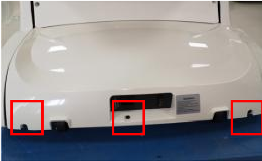
A.remove 3 screws, open the main PCB box
