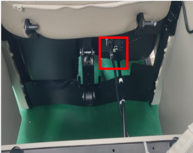
D.disconnect the terminal and air hose
