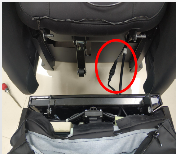
C. disconnect the terminal and air hose
