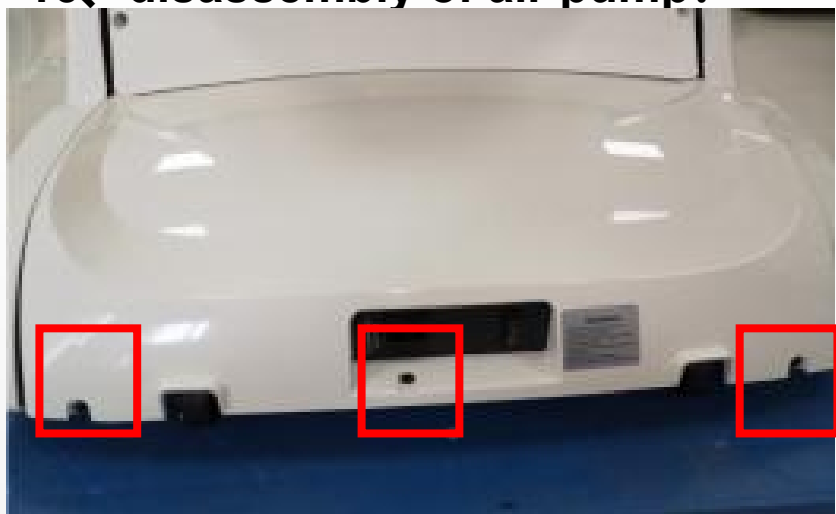
A.remove 3 screws, open themain PCB box
