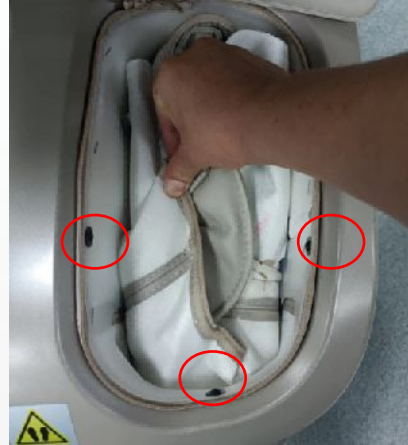
Remove 3 screws and pry out U-shaped nails
