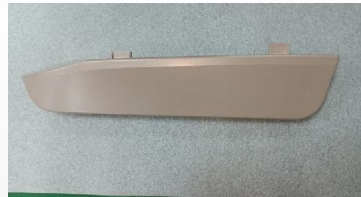
Break open the buckle and remove the armrest cover
