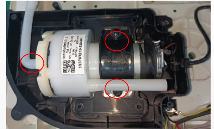
Remove 2 screws, Disconnect the air hose
