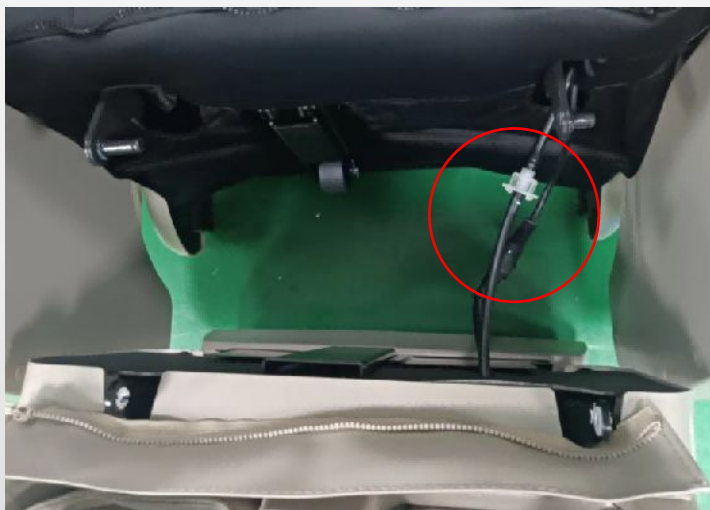
disconnect the air hose and terminals
