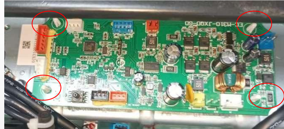
Remove the 4 Insulating column
