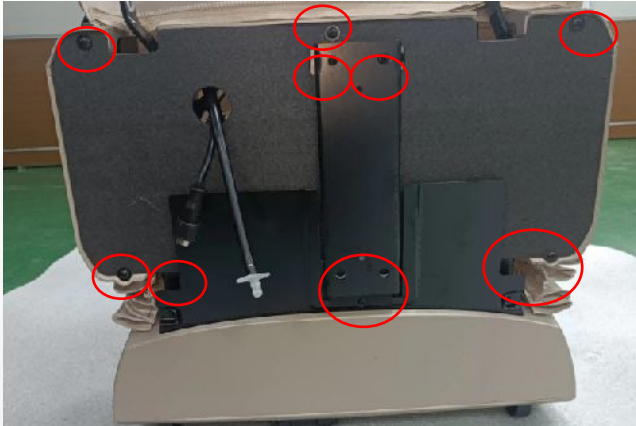
Remove 12 screws and remove the cover and hardware
