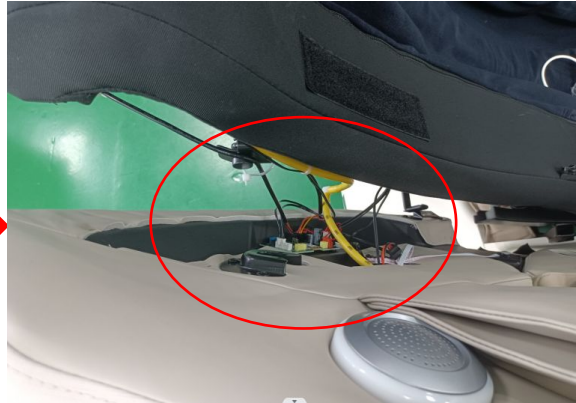
Disconnect the shoulder terminal and gas hose
