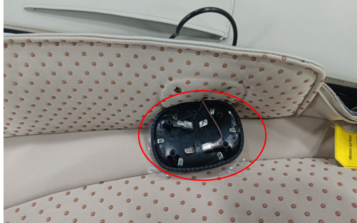
Remove 2 metal clips and uninstall the pain detection component
