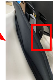
Remove 2 screws, Remove the actuator-backrest
