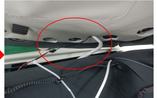
Disconnect the terminal and gas hose
