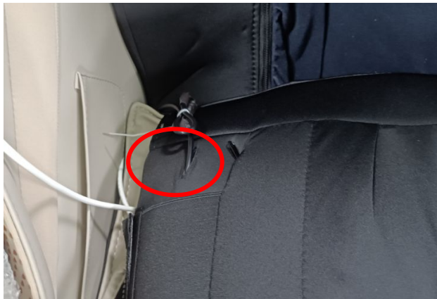
Cut off the buckle and disconnect the heating terminal
