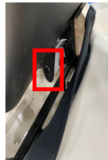
Remove 2 screws, Remove the actuator-backrest
