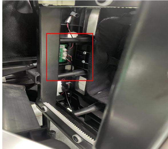
Remove 4 screws and pull out the terminal.
