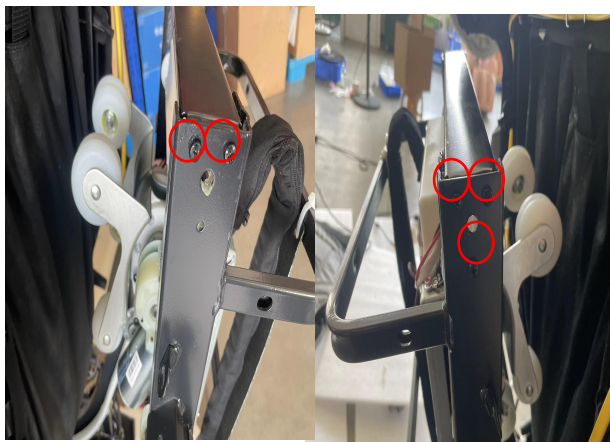
Remove 3 screws on the right and 2 screws on the left
