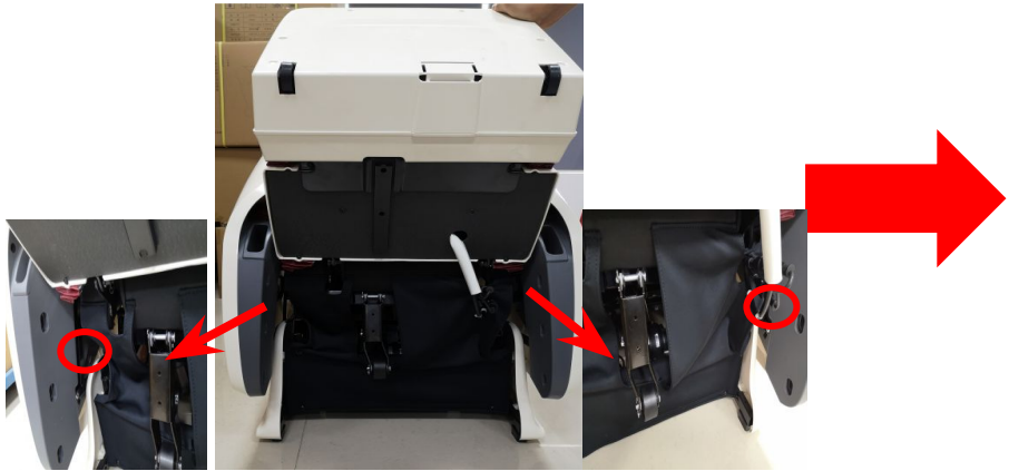
Lift up the footrest and remove 2 screws
