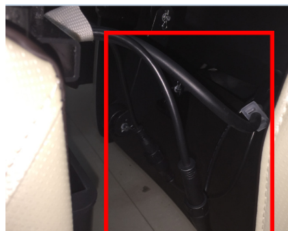
断开小腿的数据线及气管 Disconnect the 2 terminals and the air hose
