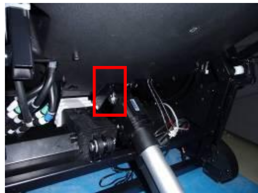
抬起小腿拆下前挡板,之后定位图中三个位置,除下它们即可(建议先拆上方销轴以方便拆底部销轴) Pull-up the legrest and disassembly the plate washer then location map of three position, (moving the top of pin first) NEXT
