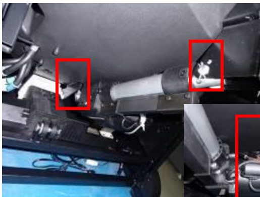
抬起小腿拆下前挡板,之后定位图中三个位置,除下它们即可(建议先拆上方销轴以方便拆底部销轴) Pull-up the legrest and disassembly the plate washer then location map of three position, (moving the top of pin first) NEXT
