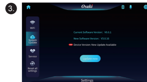
Once connected, go to "System Settings," then "Left Menu," and "System Upgrade." Wait for a minute, and check if the version number is the same. If the version number is different, it means there is a new update available. You can click the "Upgrade" button to update the tablet.
