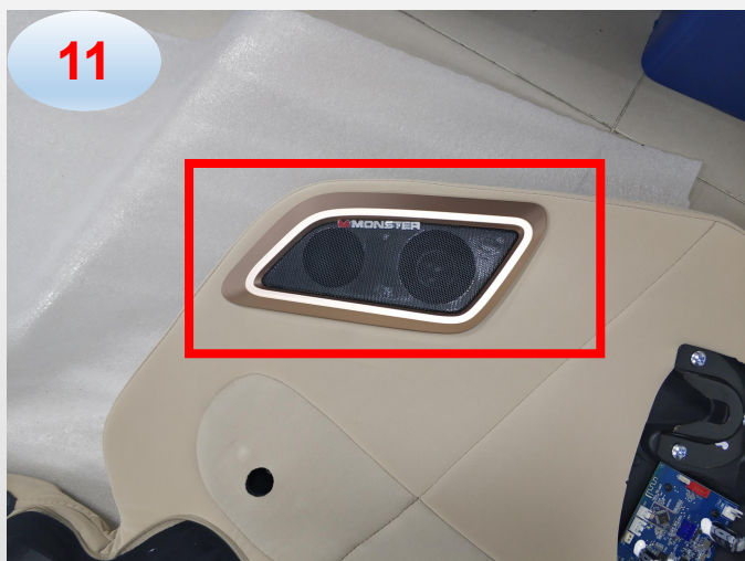
l. Tear off the horn net cover
