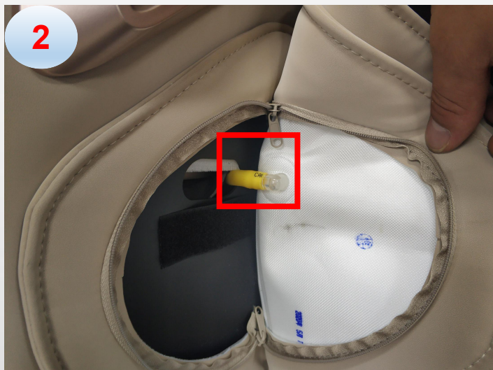
b. disconnected the air hose
