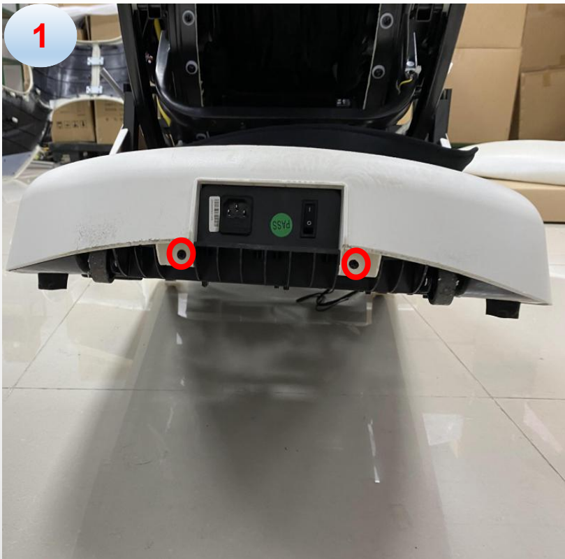
a. remove 2 screws and remove the cover
