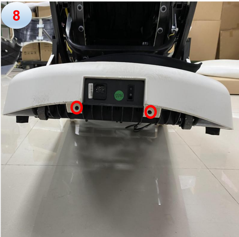
i. remove 2 screws and remove the cover
