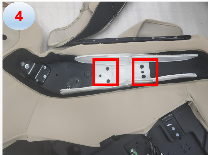
e.remove the screws, disconnected air hose, remove air bag
