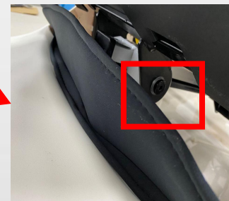
e. remove 2 screws, then remove the actuator
