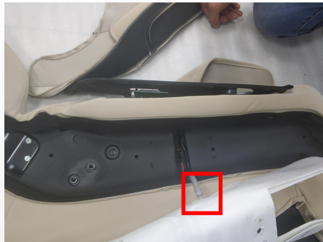
e.remove the screws, disconnected air hose, remove air bag
