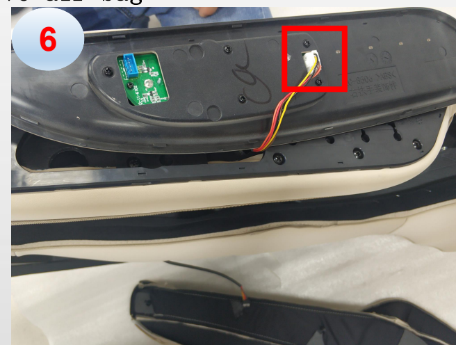
g. disconnected the terminals
