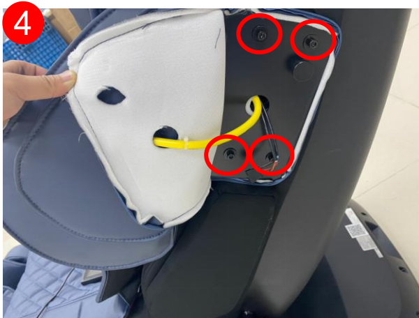
remove 4 screws, remove left shoulder unit
