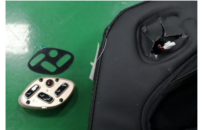
disconnected the terminal and remove the control
