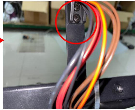
Cut off the buckle marked in green and remove the two screws marked in red
