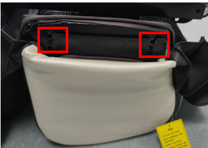
remove 2 screws both side
