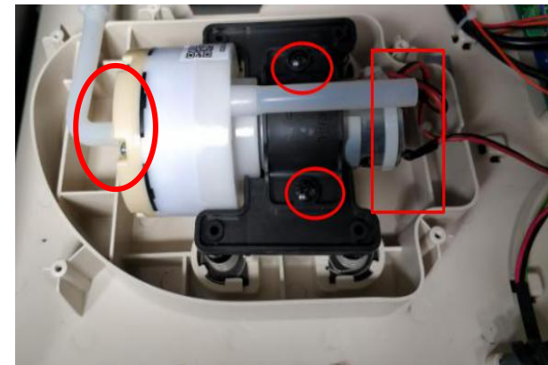
remove 2 screws, cut cable tie, remove air pump
