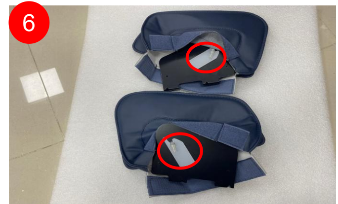
Remove the two flaps to replace the left and right side airbags and leather covers
