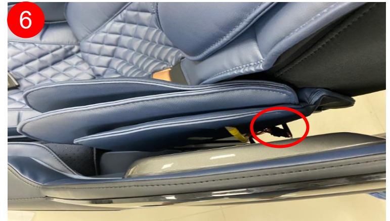
Unplug the rear horn terminal and remove the left side panel assembly
