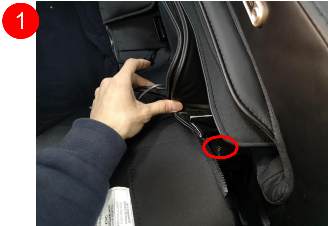
remove the screw of right side panel
