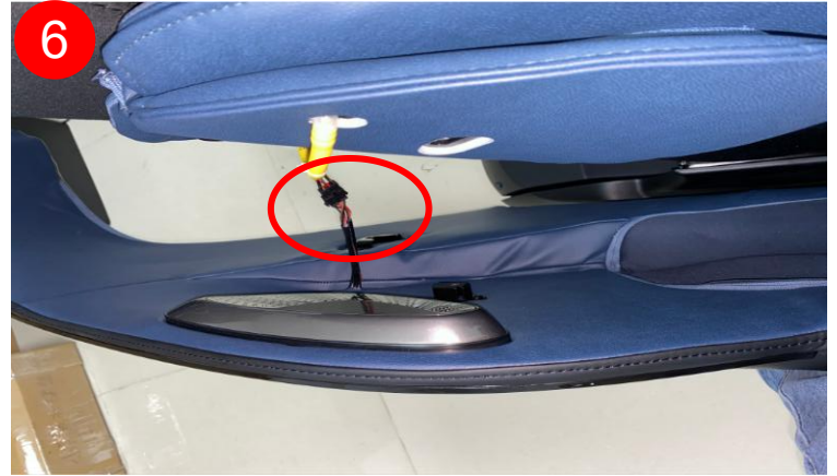
Unplug the rear horn terminal and remove the right side panel assembly
