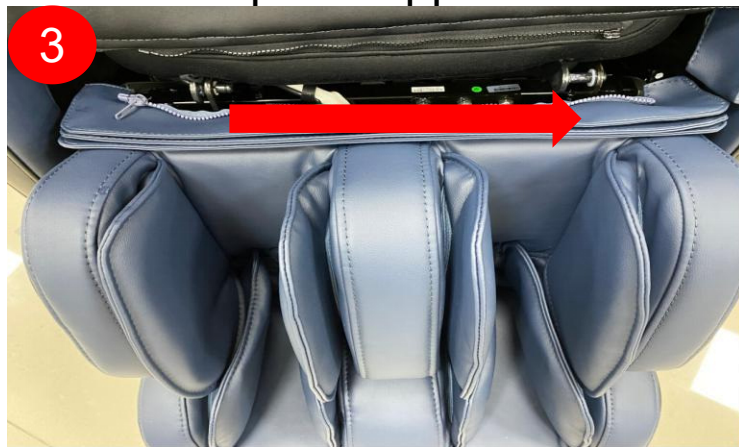
Remove the calf assembly in the direction of the arrow
