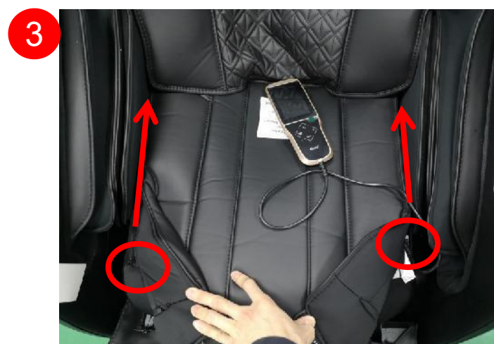
cut cable tie, reemoveheat shrinkable sleeve
