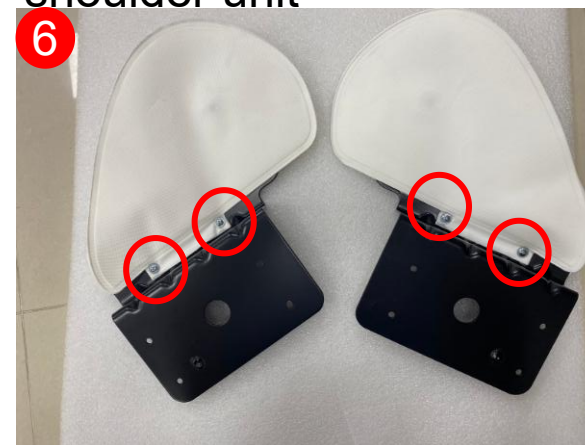
remove the screws and remove air bag
