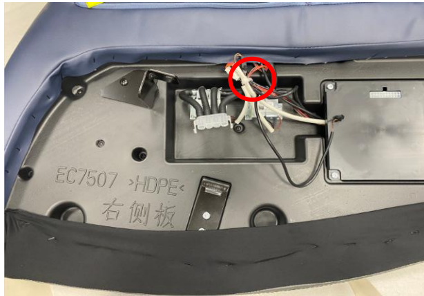
cut cable tie
