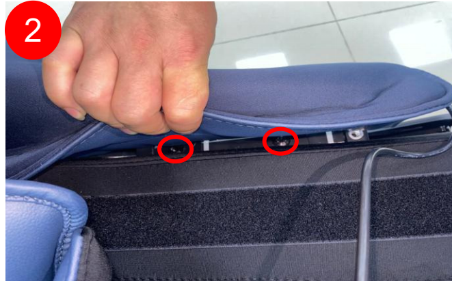
remove 2 screws, remove left side seat
