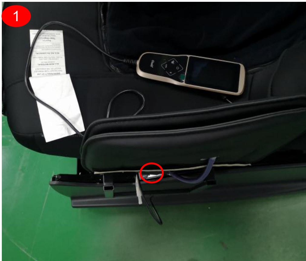
cut cable tie, discontent the terminal
