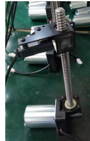
remove leg telescopic motor assembly
