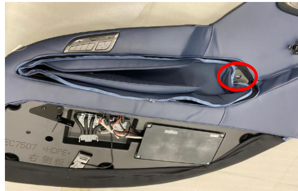
the cloth cover pin can be directly pulled out
