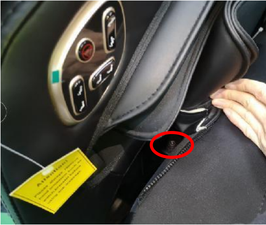
remove the screw of right side panel
