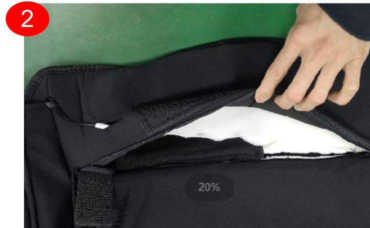
discontent terminals, remove heater
