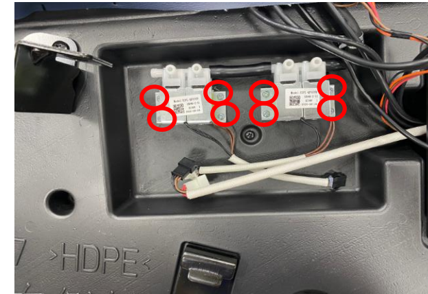
remove 8 screws, remove air valves
