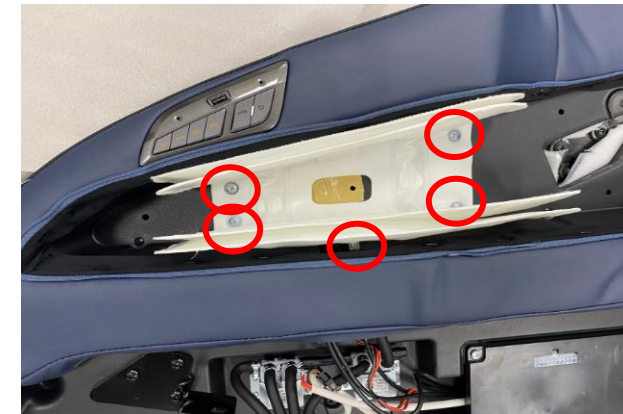
remove 4 screws and remove air bag
