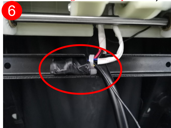
cut the heat shrinkable sleeve
