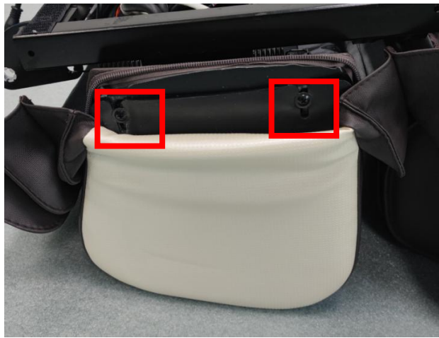
disconnected air hose and terminal, unzip the zipper
