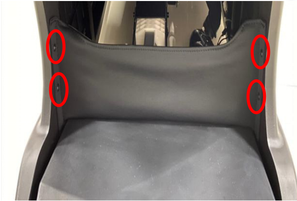
disassemble the cloth block
