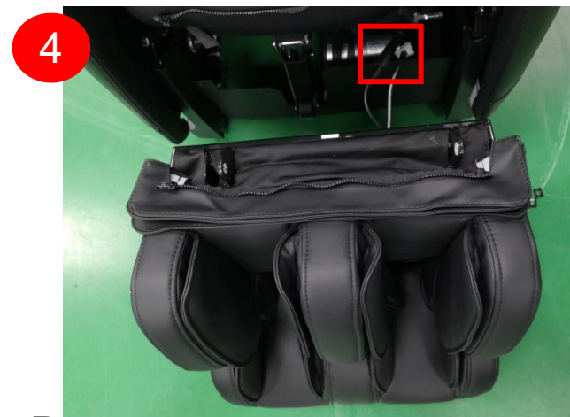
Pull out the terminal and air hose, pull out the pin and pin shaft, and take out the leg assembly
