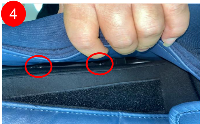
remove 2 screws, remove right side seat
