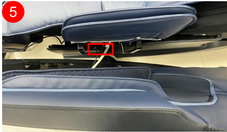
cut cable, discontent terminal and air hose
