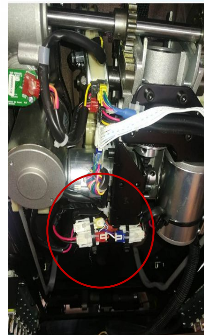
4. Cut the cable tie, unscrew the bolt and unplug it, then take out whole Mech.
