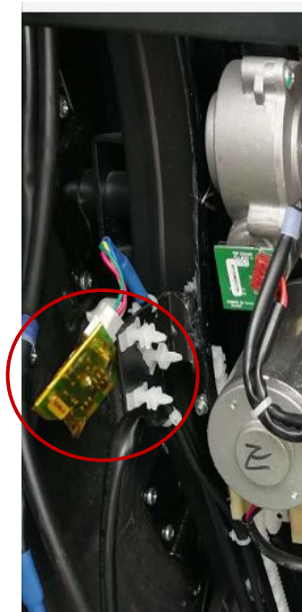
2. Take off the Upper Limit Sensor Detection Board, but do not unplug it.
