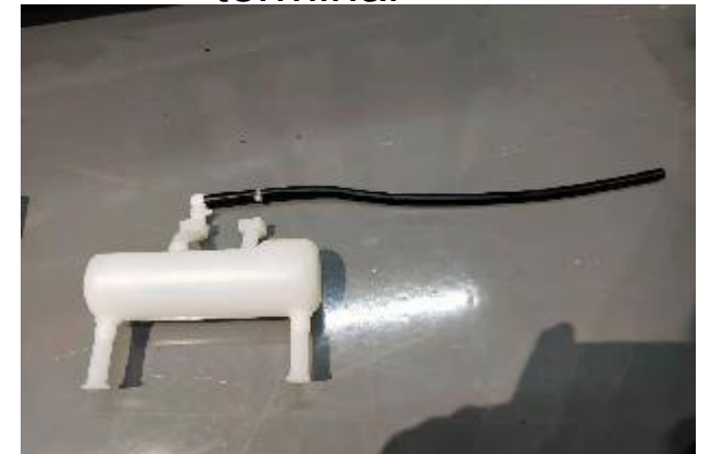
C.disconnect the air hose and terminal
