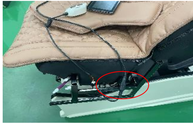
E. disconnected the terminal
