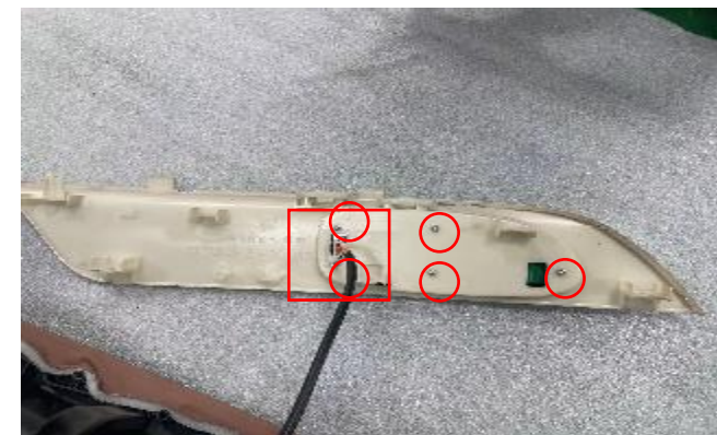
F.remove 5 screws, discontent the tterminal
