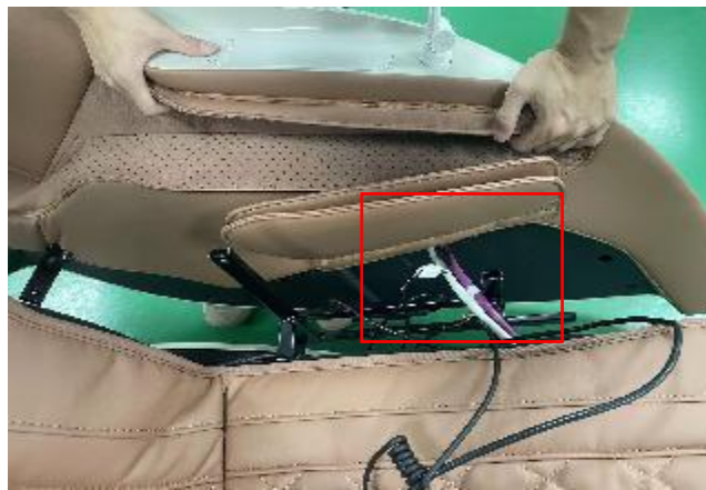
B. discontent the terminal and air hose
