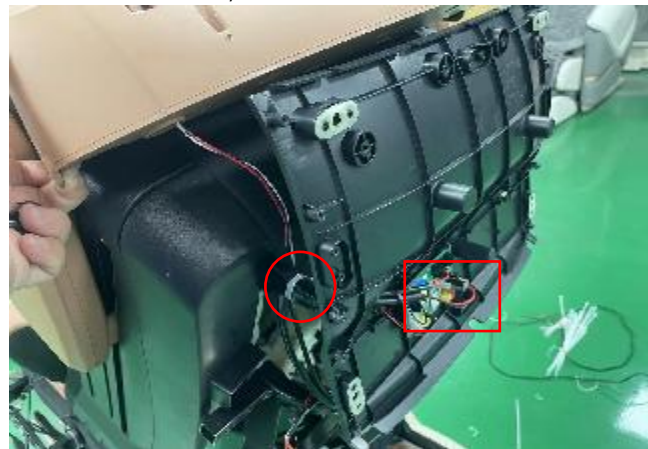
E.cut the cable tie, discontent 2 terminals
