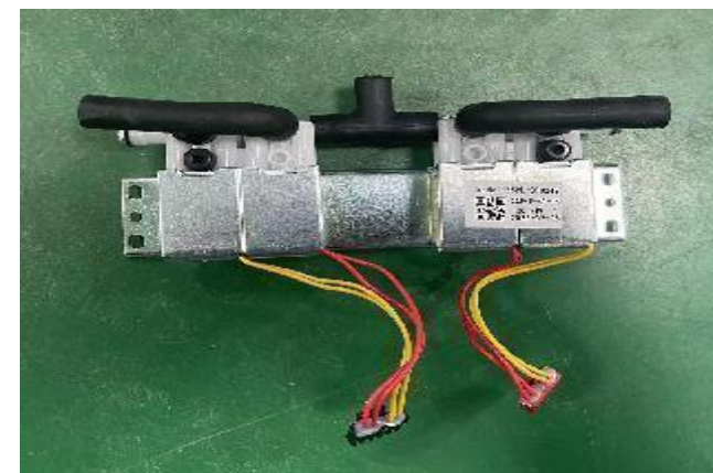
L.remove the air valve
