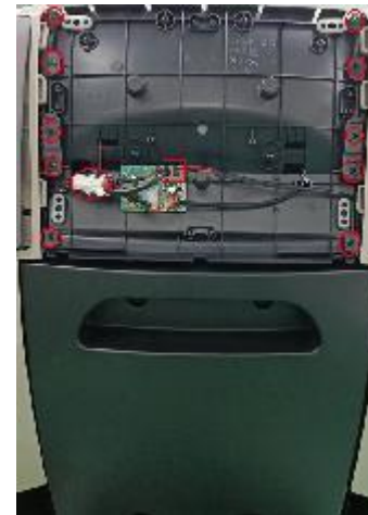
C.Disconnect the port and remove 10 screws
