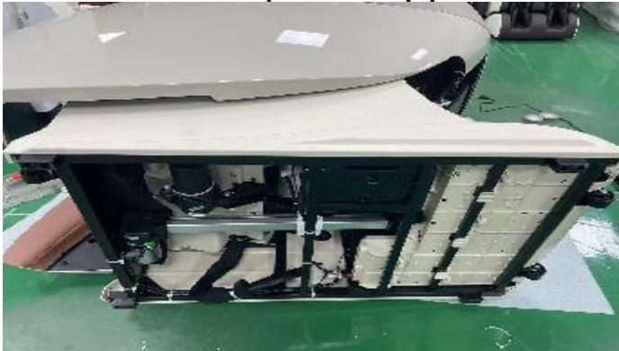
D.The chair should fall to the right. Pay attention to prevent the side panel trim from being scratched
