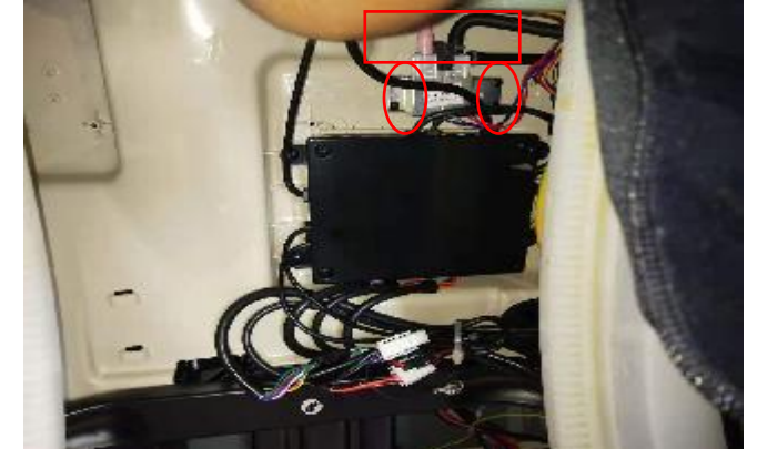
C.remove the screws, disconnect the terminals, remove air valve
