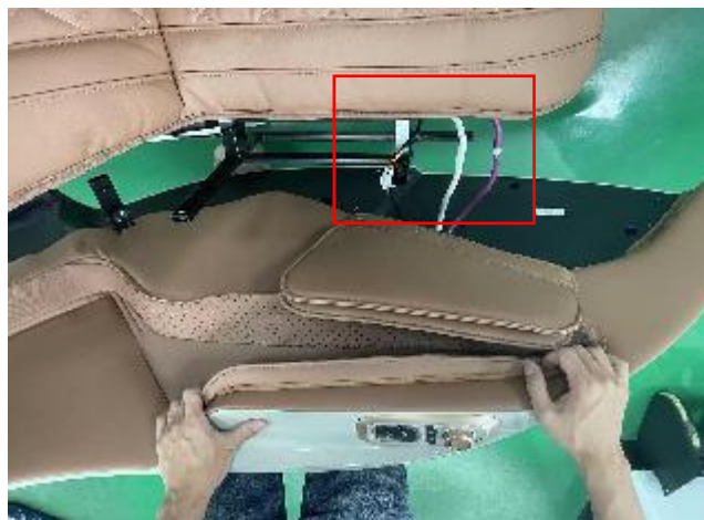
E. discontent the terminal and air hose
