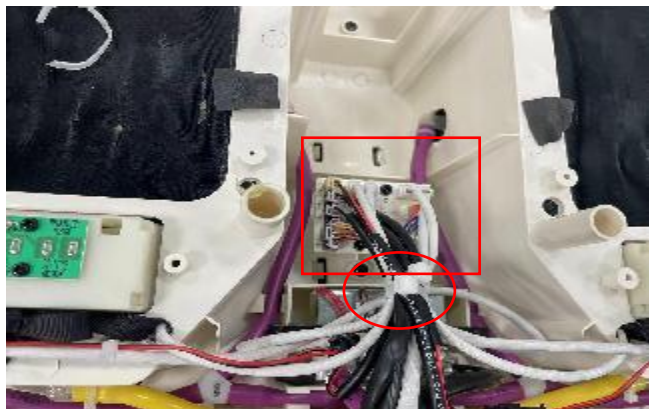
G.cut cable tie, discontent the terminals
