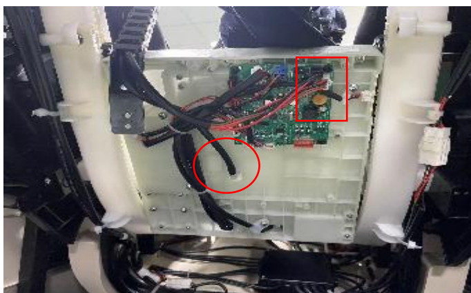
D.discontent 1 air hose, 2 terminals
