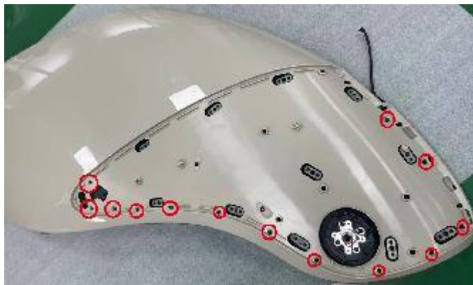
B. remove 13 screws
