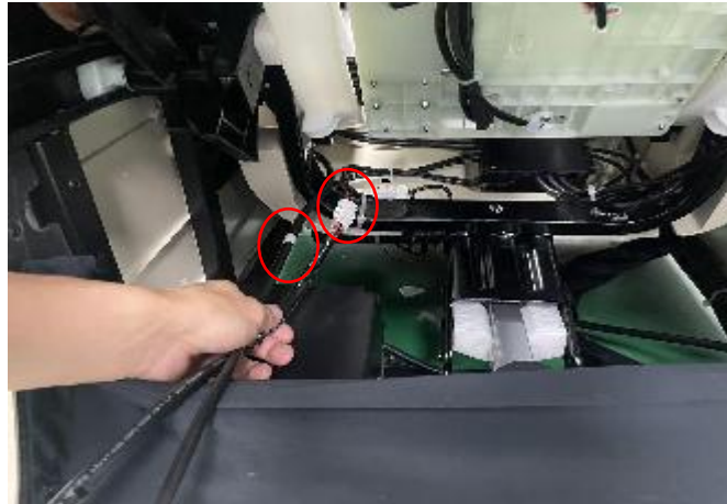
H.disconnect the terminal and air hose
