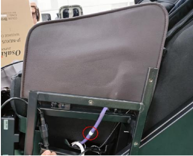
1 Disconnect the air hose interface
