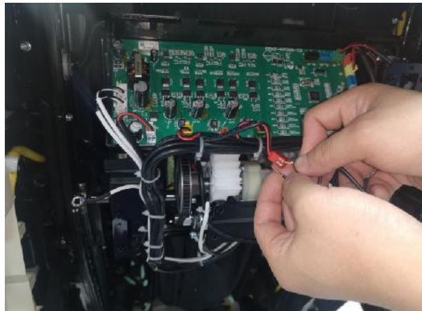
4 Connect the red terminal to an external 24V power supply to move the gear box up and down for removal
