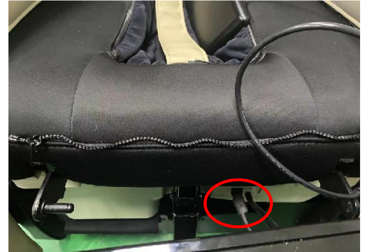
3.disconnect the terminal and air hose
