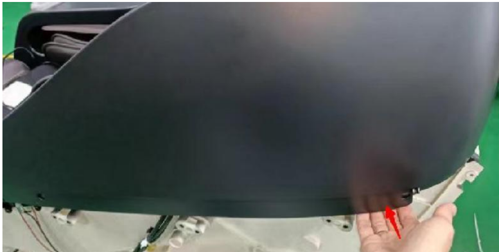
4. Pull apart the left front side panel cover and left upper side panel cover
