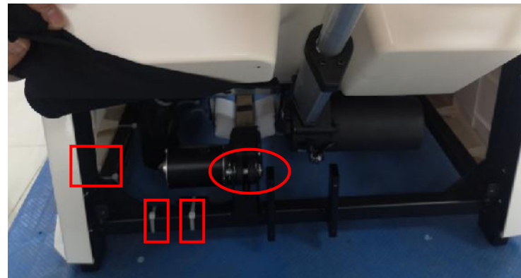
E.cut cable, remove the shaft
