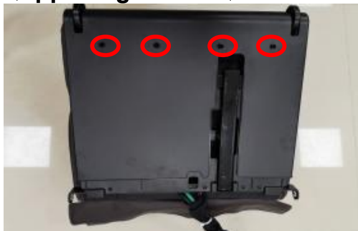
remove 4 screws take down the cover
