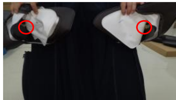
disconnect the air hose and take down the shoulder massage
