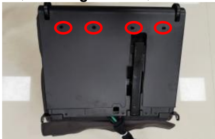
remove 4 screws take down the cover
