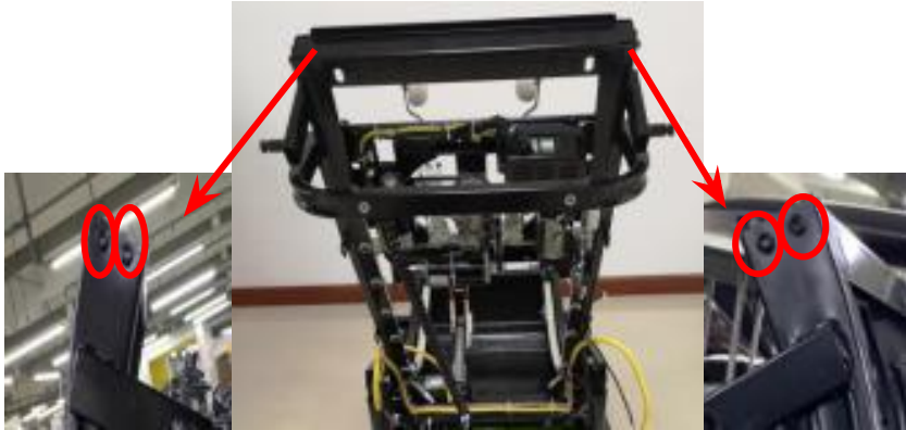
remove 4 screws, take down the frame
