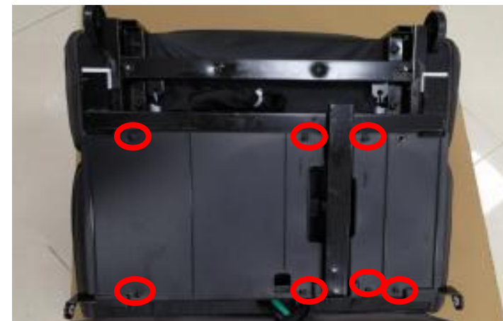
remove 7 screws and take down the cover
