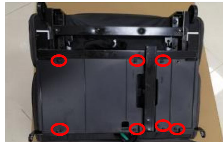
remove 7 screws and take down the cover
