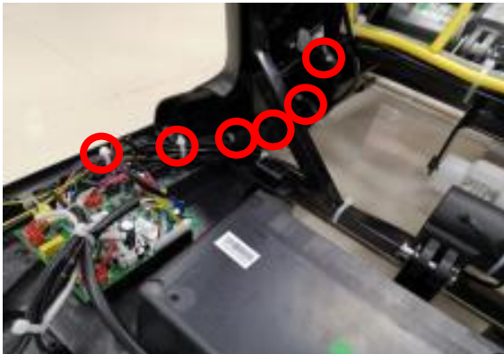
cut the cable tie
