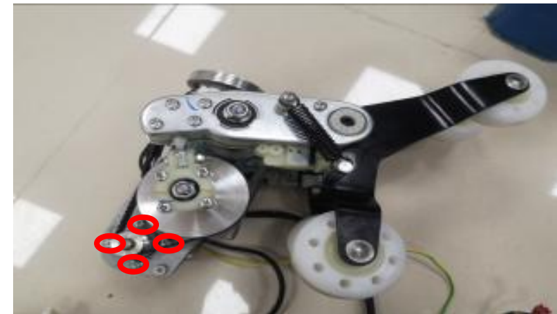
remove 4 screws and take down tapping motor
