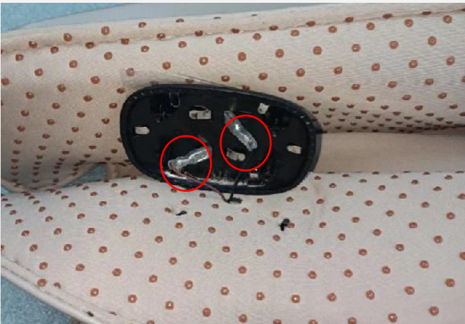
disconnect the signal terminal
