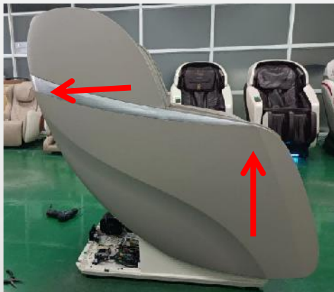
Lift the side panel up first, then move it back out
