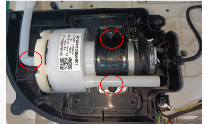
Remove 2 screws, Disconnect the air hose
