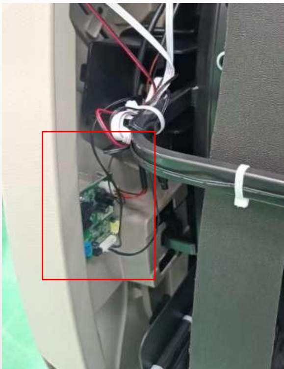
disconnect the signal terminal
