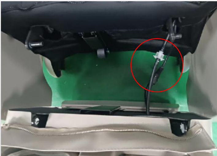
disconnect the air hose and terminals
