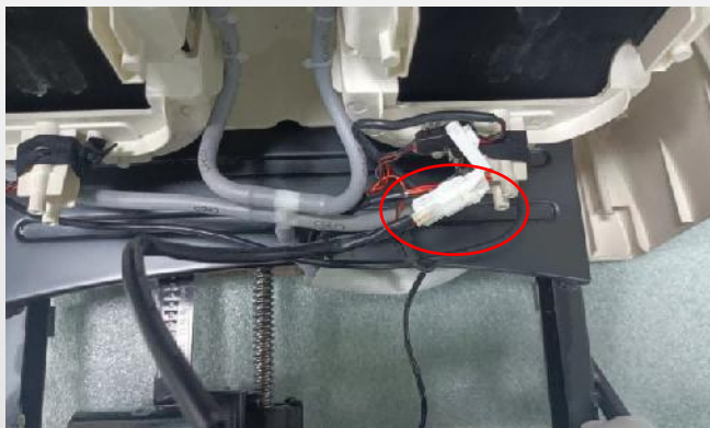
Cut off the buckle and disconnect the signal terminal
