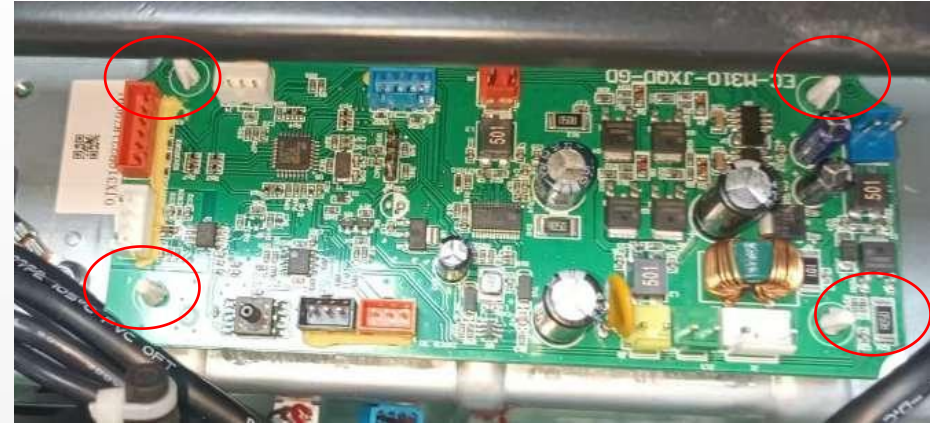
Remove the 4 Insulating column
