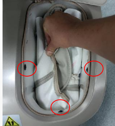
Remove 3 screws and pry out U-shaped nails
