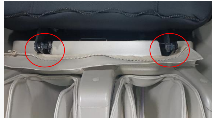
remove 2 limit baffles
