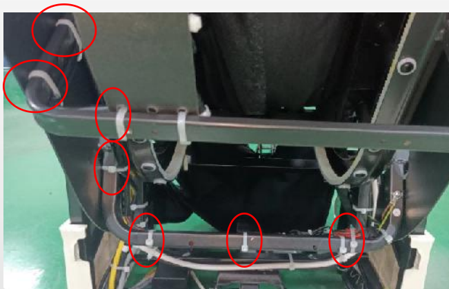
Cut off the buckle and disconnect the signal terminal
