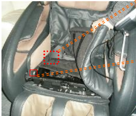
Screws (2pcs) securing the front panel
