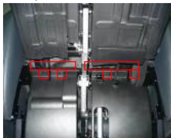
Screws(12pcs) securing the front panel
