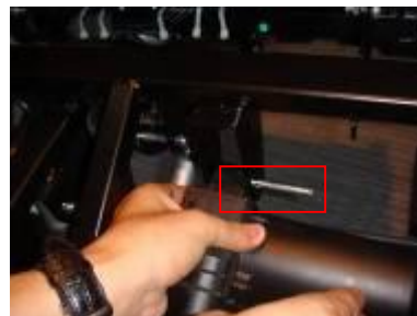
Flat head rivet securing the reclining actuator on the U stay fork
