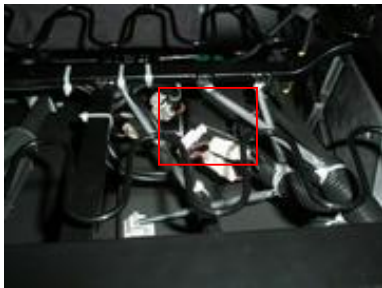
Connectors of the wires of foot rest
