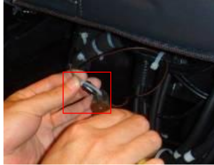
Cable ties tightening the wire and connector
