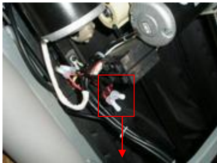
Close-end wire connector of tapping motor
