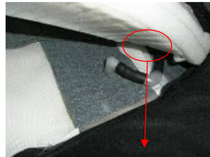
Pull out the hoses
