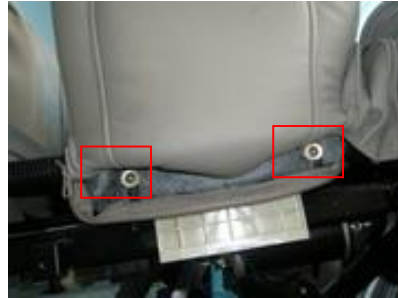
Screws fixing the outer coating
