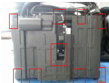
Screws(9PCS) fixing the cover of footrest
