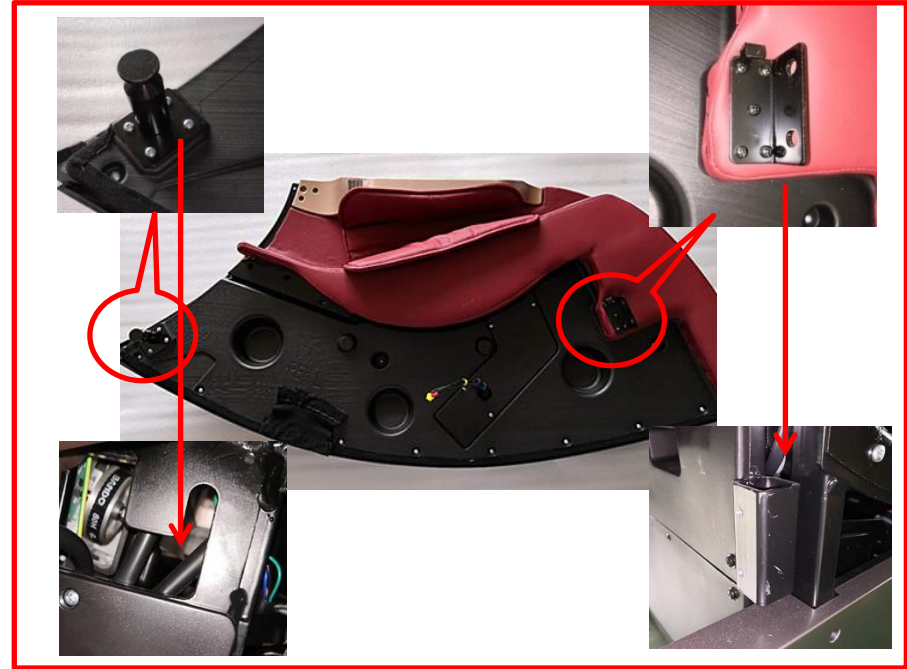
B、 Install the front and rear ends of armrest and fix two screws at front.
