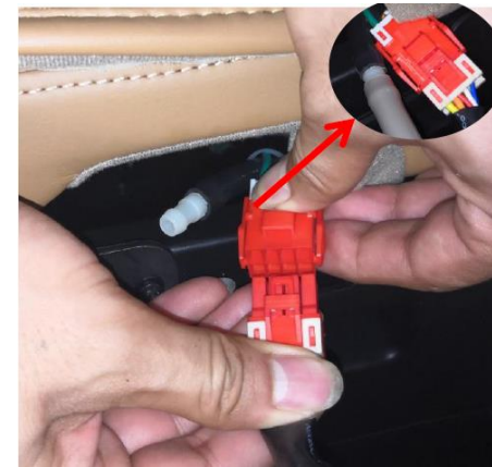
C、 Secure harness and air pipe
