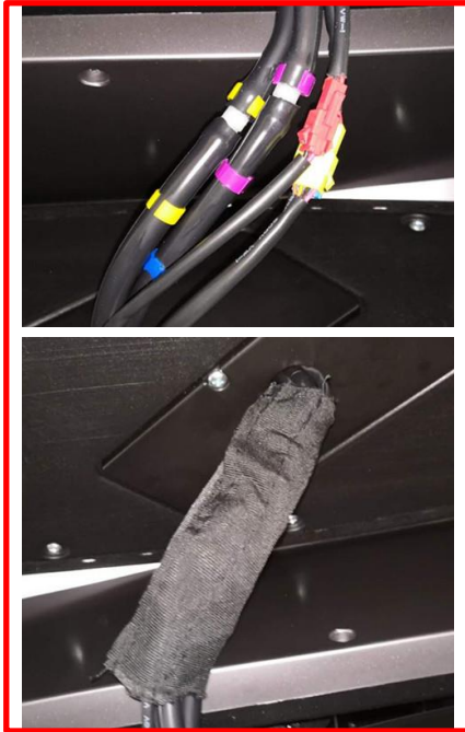
A、 Connect air pipe and harness, set protective cover
