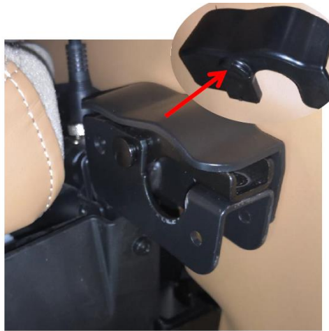
A、 Remove the cover on both sides of calf
