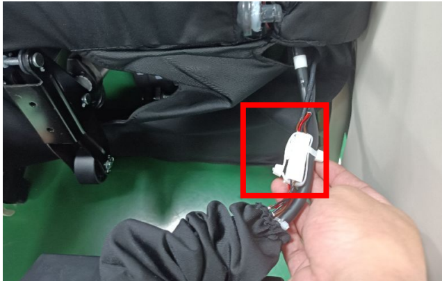
Cut off the buckle, pull out the terminal and air pipe.
