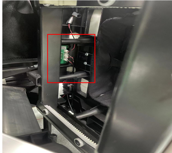
Remove 4 screws and pull out the terminal.
