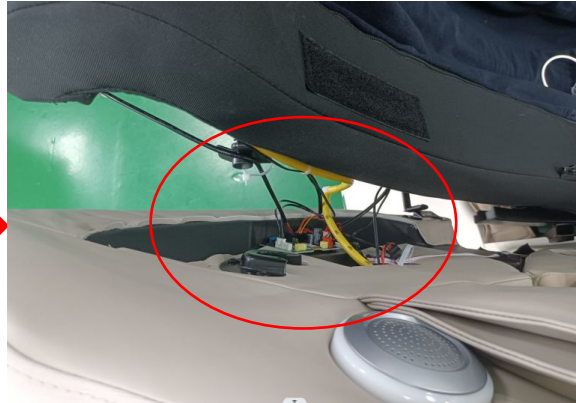
Disconnect the shoulder terminal and gas hose
