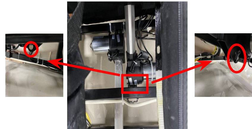
Pull out the socket and pin, and remove the actuator-legrest
