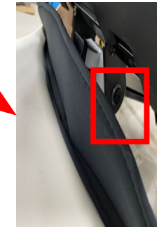
Remove 2 screws, Remove the actuator-backrest
