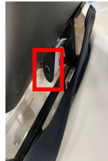
Remove 2 screws, Remove the actuator-backrest
