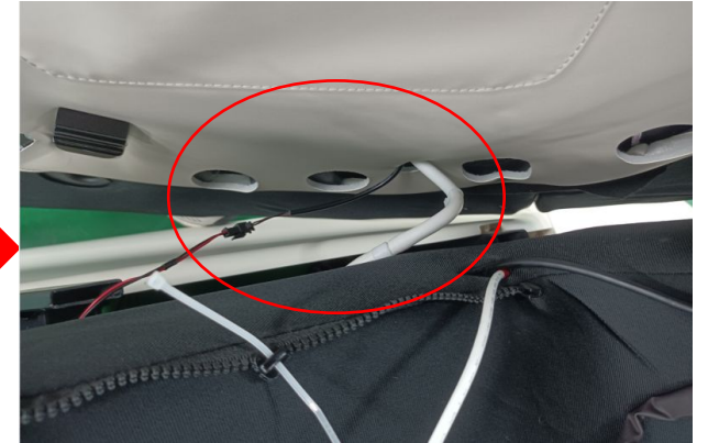
Disconnect the terminal and gas hose
