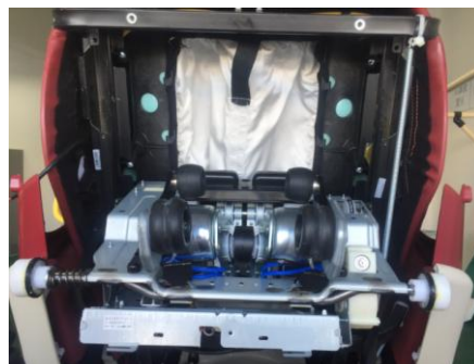
转动行走电机，直到机芯可以脱离背架 Turn motor, until the movement can be separated from the back
