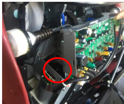
转动行走电机，直到机芯可以脱离背架 Turn motor, until the movement can be separated from the back
