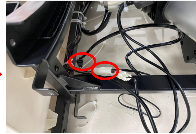
Disconnect the two terminals
