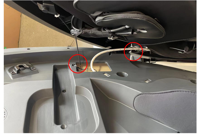
Disconnect the terminal and air pipe
