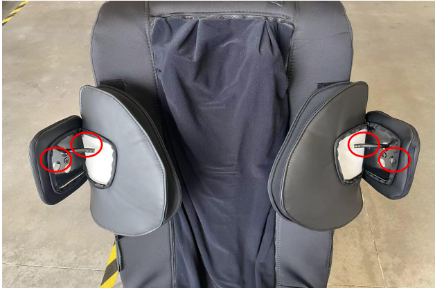
Remove 2 screws and disconnect the air pipe
