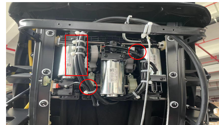
cut the cable ties remove 4 screws
