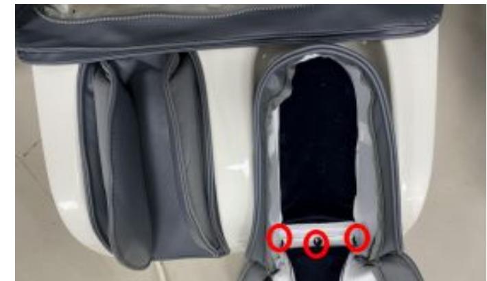
Remove the 3 screws and remove the holster
