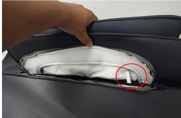
Remove the air bag and cut the tie to disconnect the trachea
