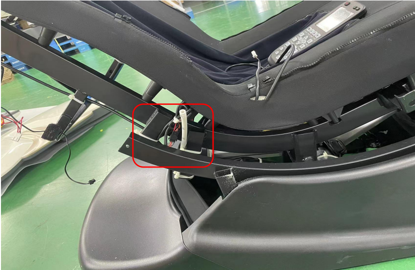
Cut off the cable tie and unplug one terminal
