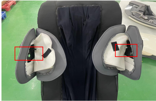
Tear open the magic buckle and remove it (2 screws on each side)
