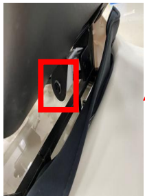
Remove 2 hex screws and remove the backrest push rod
