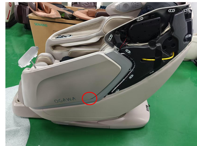
Remove the left decorative piece (remove the right side as the left side)
