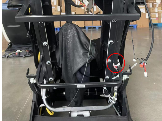
Cut off the backrest wire cable tie
