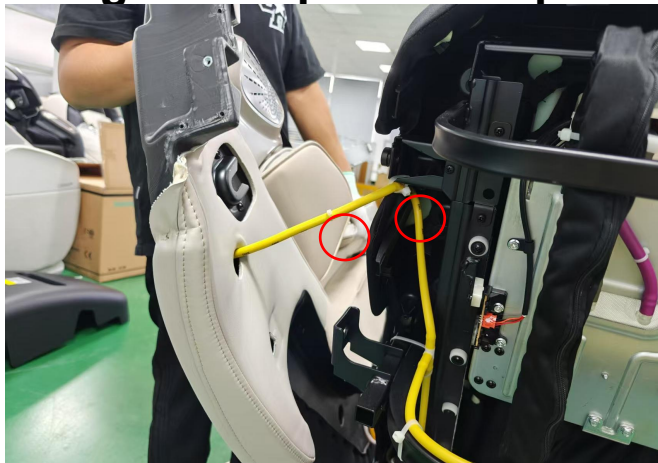
Lift the side panel upwards, cut off the zip ties, and remove the trachea
