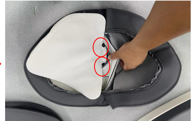
Remove the two screws on the right shoulder
