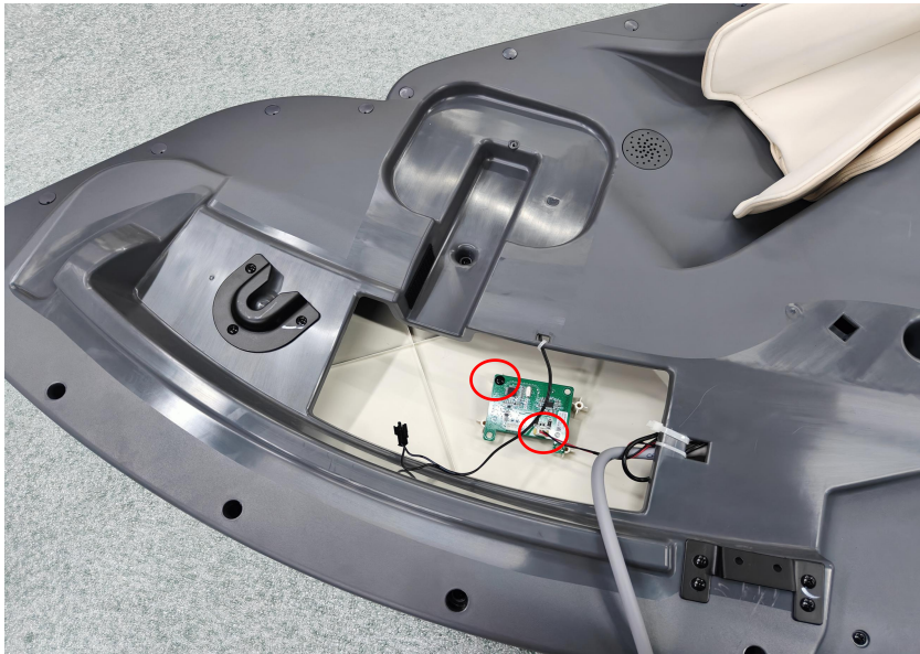
Remove one screw and disconnect one terminal
