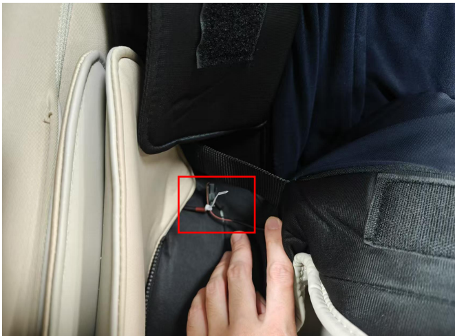
Cut off the zip ties and heat shrink tubing
