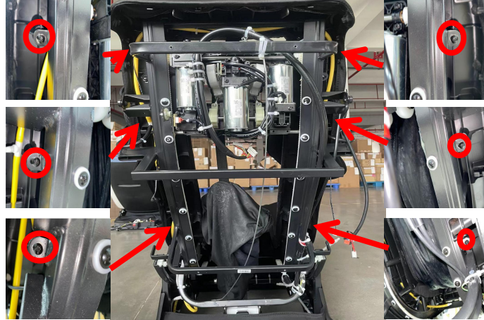
Remove the 6 screws securing the front backrest
