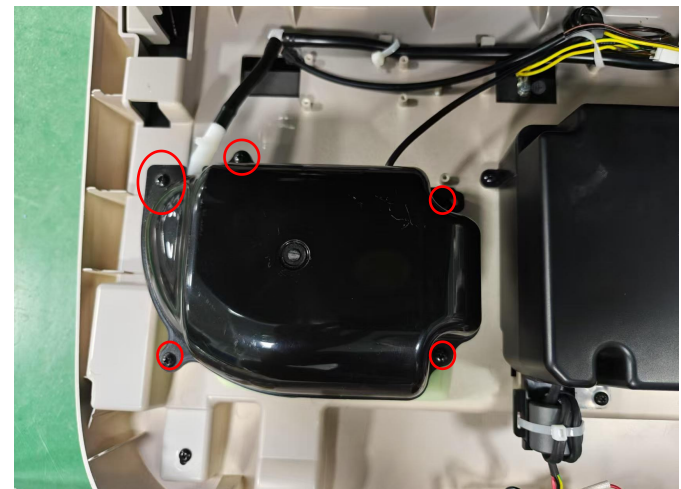
Remove 5 screws and take off the cover
