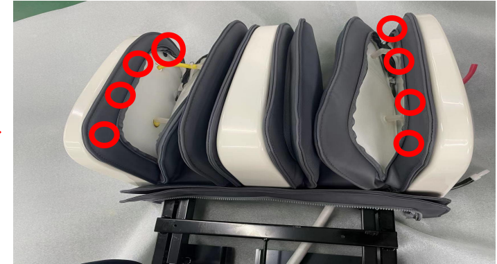
Remove a total of 8 screws on the left and right sides
