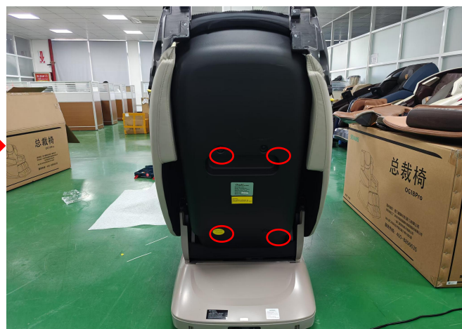
Remove the four screws and remove the backrest back cover
