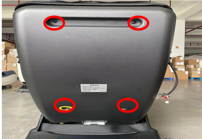
Remove 4 screws and take off the backrest back cover
