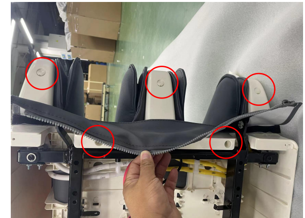
Pick out 3 plugs and remove 5 screws
