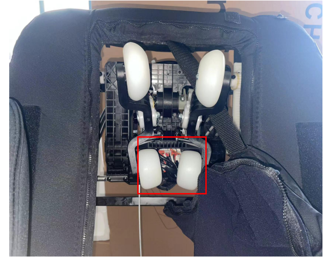
Remove all terminals from the adapter board of the movement
