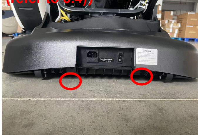
Remove 2 screws and take off the top cover of the center box
