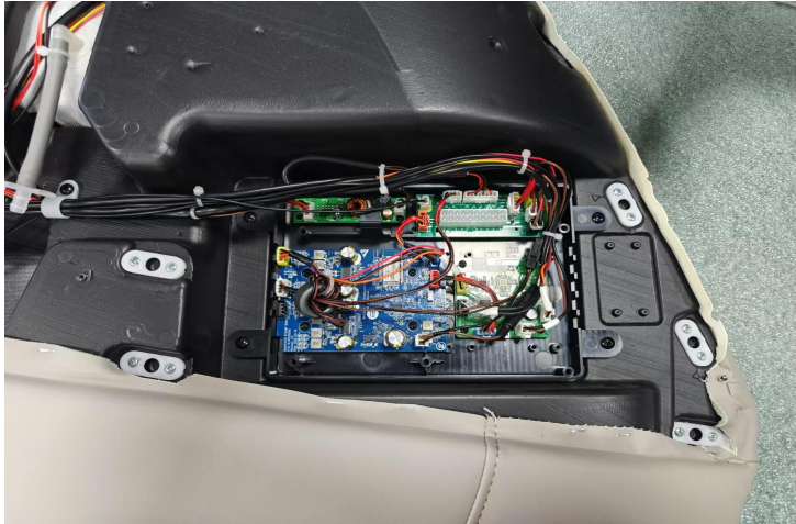
Remove 4 cross screws from 4 boards and unplug the terminals
