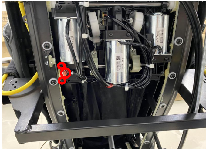
Remove 2 screws and unplug the terminals
