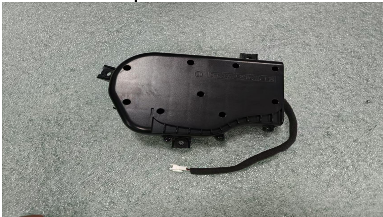
Remove the horn component
